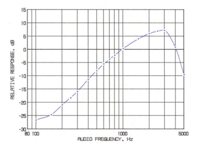
MODULATION FREQUENCY RESPONSE FCC ID: MMAG15
