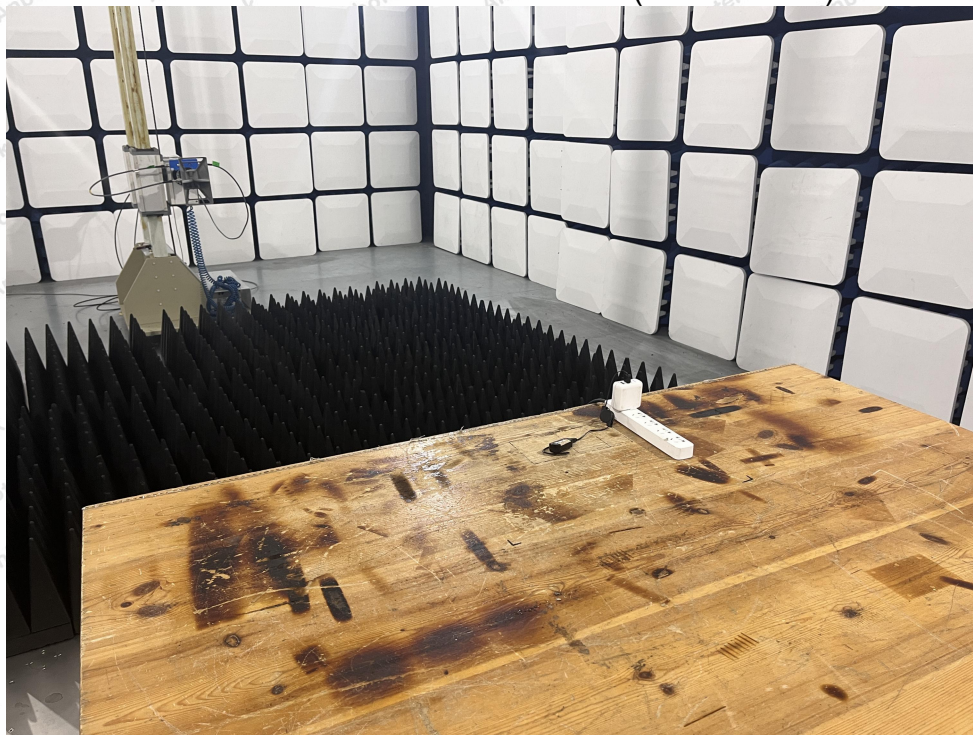
Photo of Radiation Emission Test (Above 1GHz)
