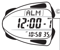
Alarm on indicator
