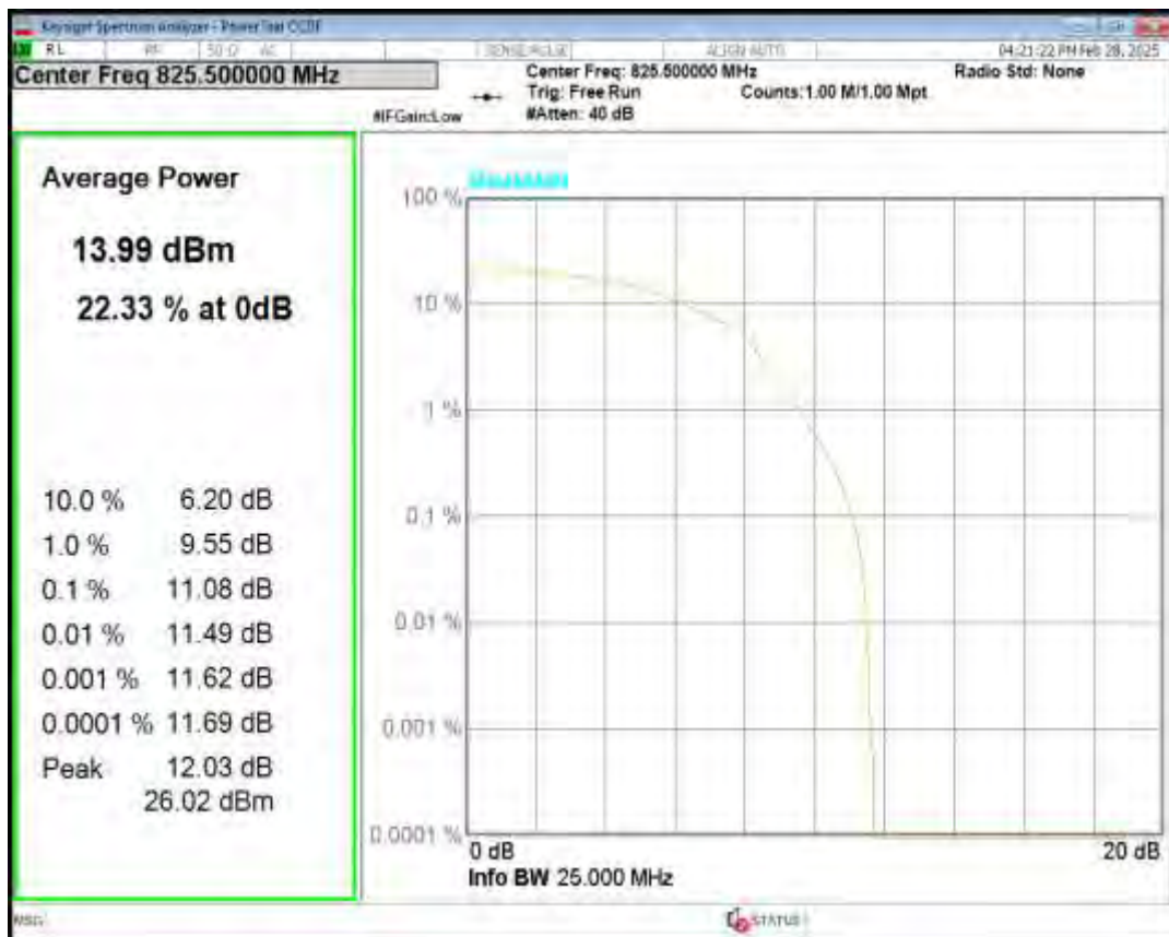
Band26(824-849) QPSK BW=3MHz Channel=26915 RB Size=6 Position=#0 NB Index=0
