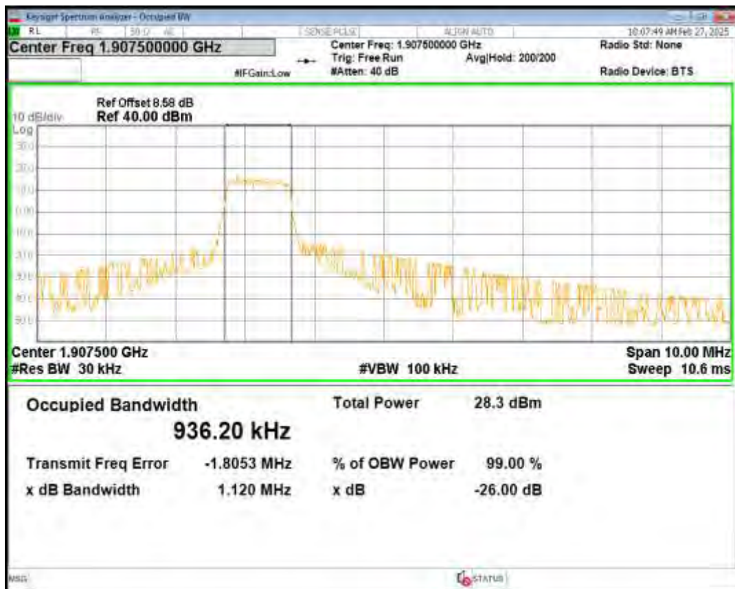
Band2 QPSK BW=10MHz Channel=18650 RB Size=6 Position=#0 NB Index=0
