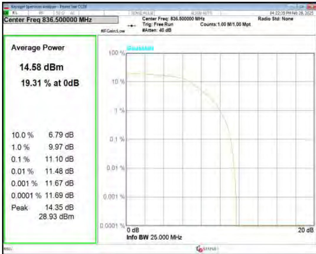
Band26(824-849) 16QAM BW=15MHz Channel=26915 RB Size=5 Position=#0 NB Index=0
