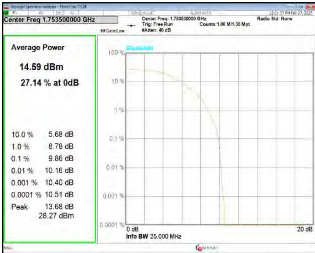
Band4 16QAM BW=3MHz Channel=20385 RB Size=5 Position=#0 NB Index=0
