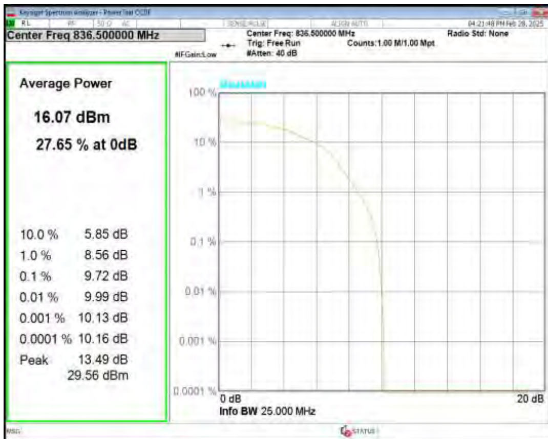
Band26(824-849) QPSK BW=5MHz Channel=27015 RB Size=6 Position=#0 NB Index=0
