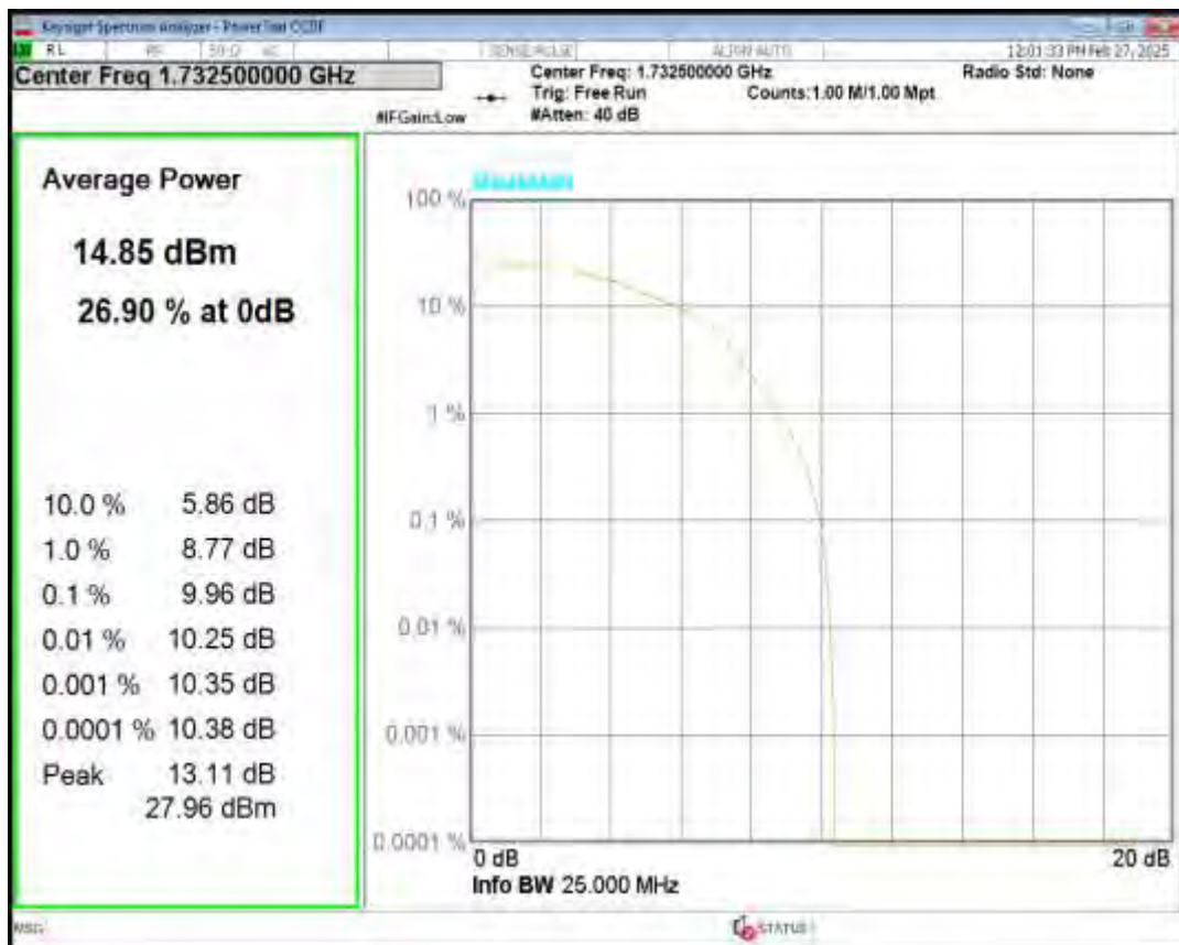
Band4 QPSK BW=3MHz Channel=20385 RB Size=6 Position=#0 NB Index=0
