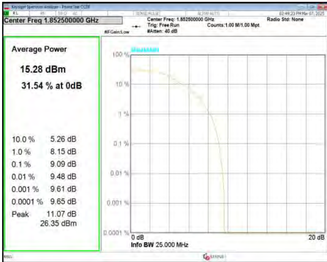
Band25 16QAM BW=5MHz Channel=26065 RB Size=5 Position=#0 NB Index=0
