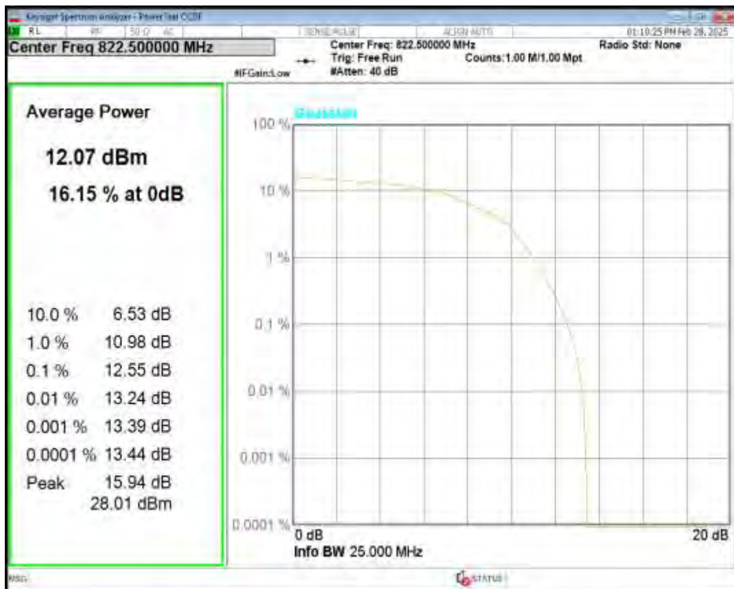
Band26(814-824) QPSK BW=5MHz Channel=26715 RB Size=6 Position=#0 NB Index=0
