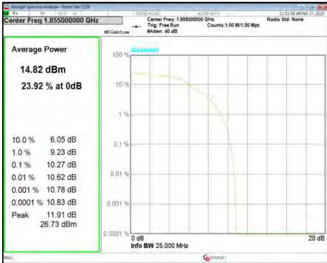
Band2 16QAM BW=10MHz Channel=18650 RB Size=5 Position=#0 NB Index=0
