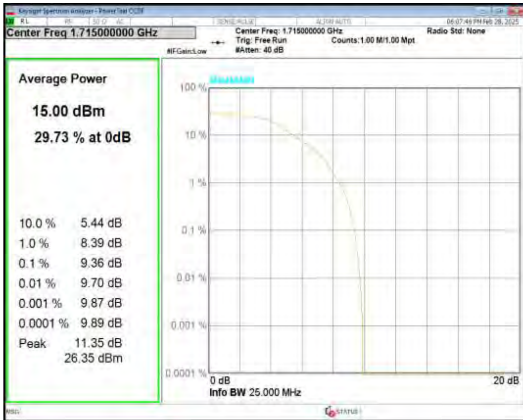
Band66 16QAM BW=10MHz Channel=132022 RB Size=5 Position=#0 NB Index=0
