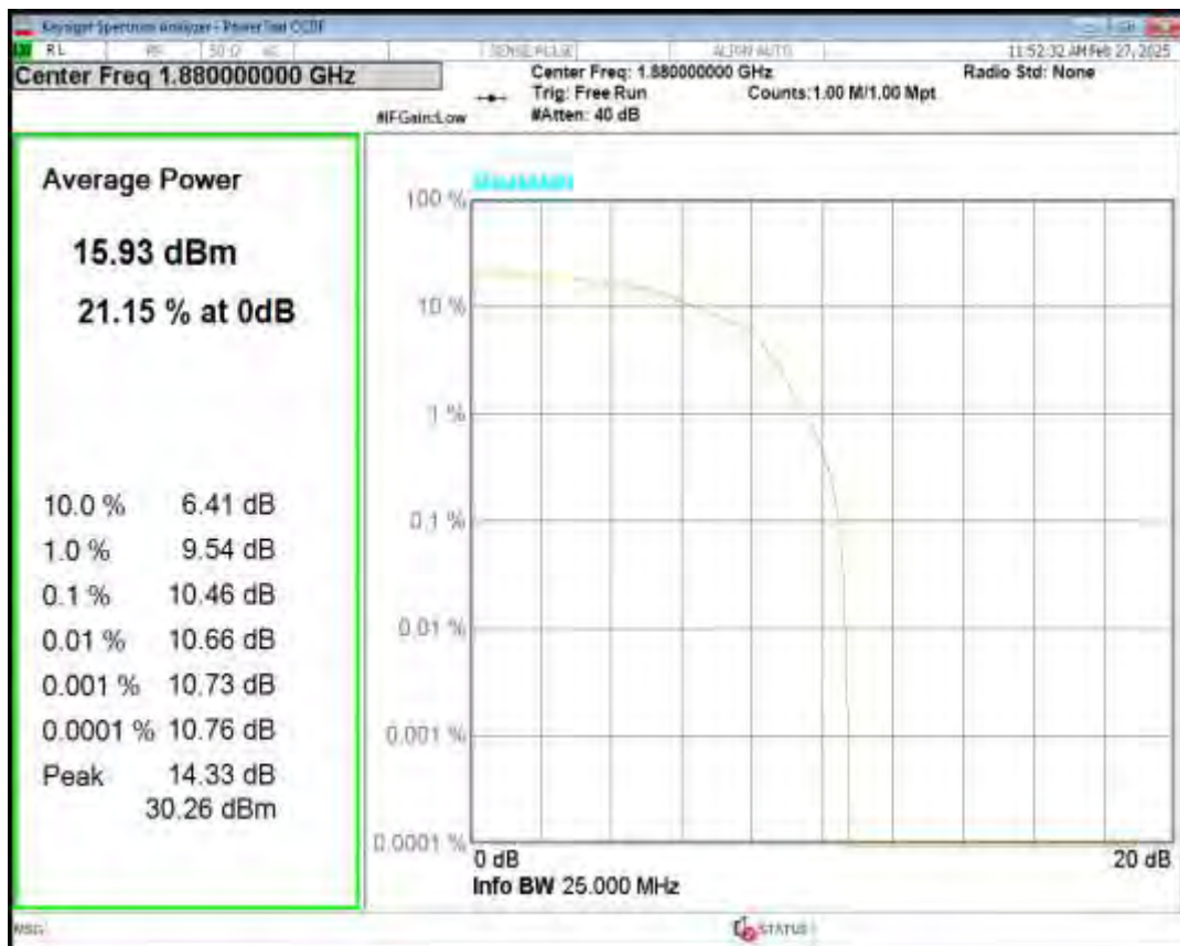
Band2 QPSK BW=15MHz Channel=19125 RB Size=6 Position=#0 NB Index=0
