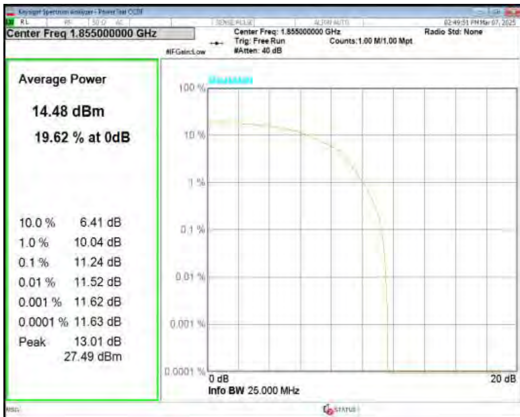
Band25 QPSK BW=10MHz Channel=26365 RB Size=6 Position=#0 NB Index=0
