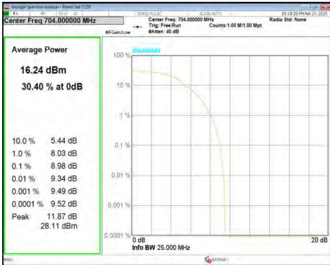
Band12 16QAM BW=10MHz Channel=23060 RB Size=5 Position=#0 NB Index=0
