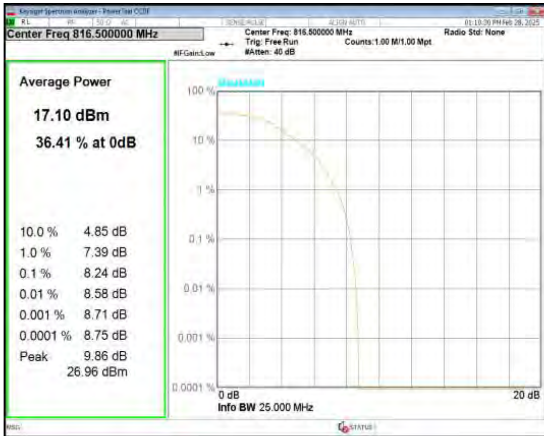
Band26(814-824) 16QAM BW=5MHz Channel=26715 RB Size=5 Position=#0 NB Index=0
