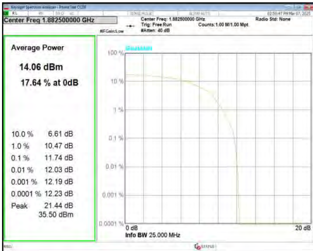
Band25 QPSK BW=20MHz Channel=26590 RB Size=6 Position=#0 NB Index=0
