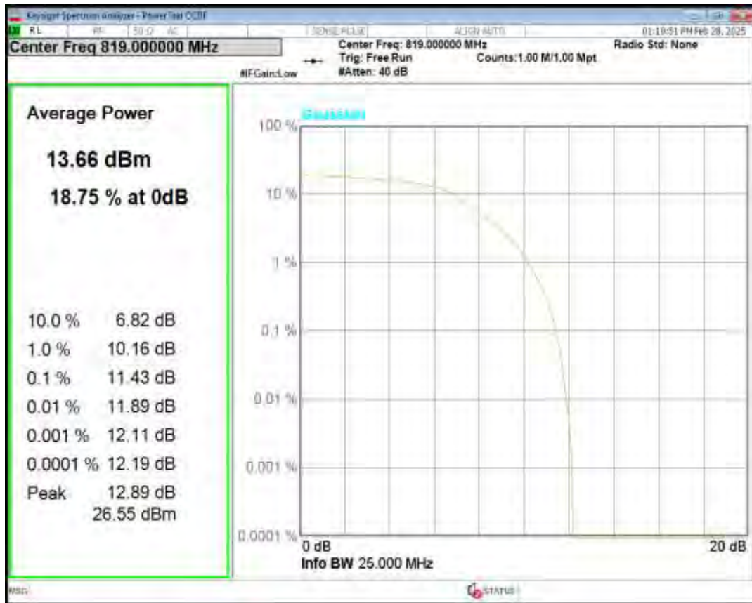
Band26(814-824) 16QAM BW=10MHz Channel=26740 RB Size=5 Position=#0 NB Index=0
