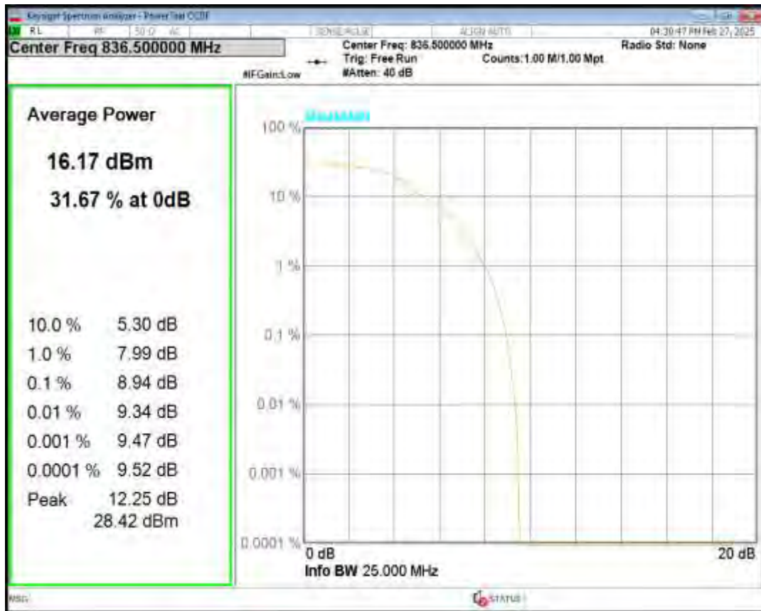
Band5 16QAM BW=5MHz Channel=20525 RB Size=5 Position=#0 NB Index=0
