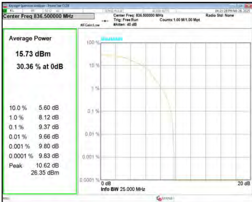
Band26(824-849) QPSK BW=3MHz Channel=27025 RB Size=6 Position=#0 NB Index=0
