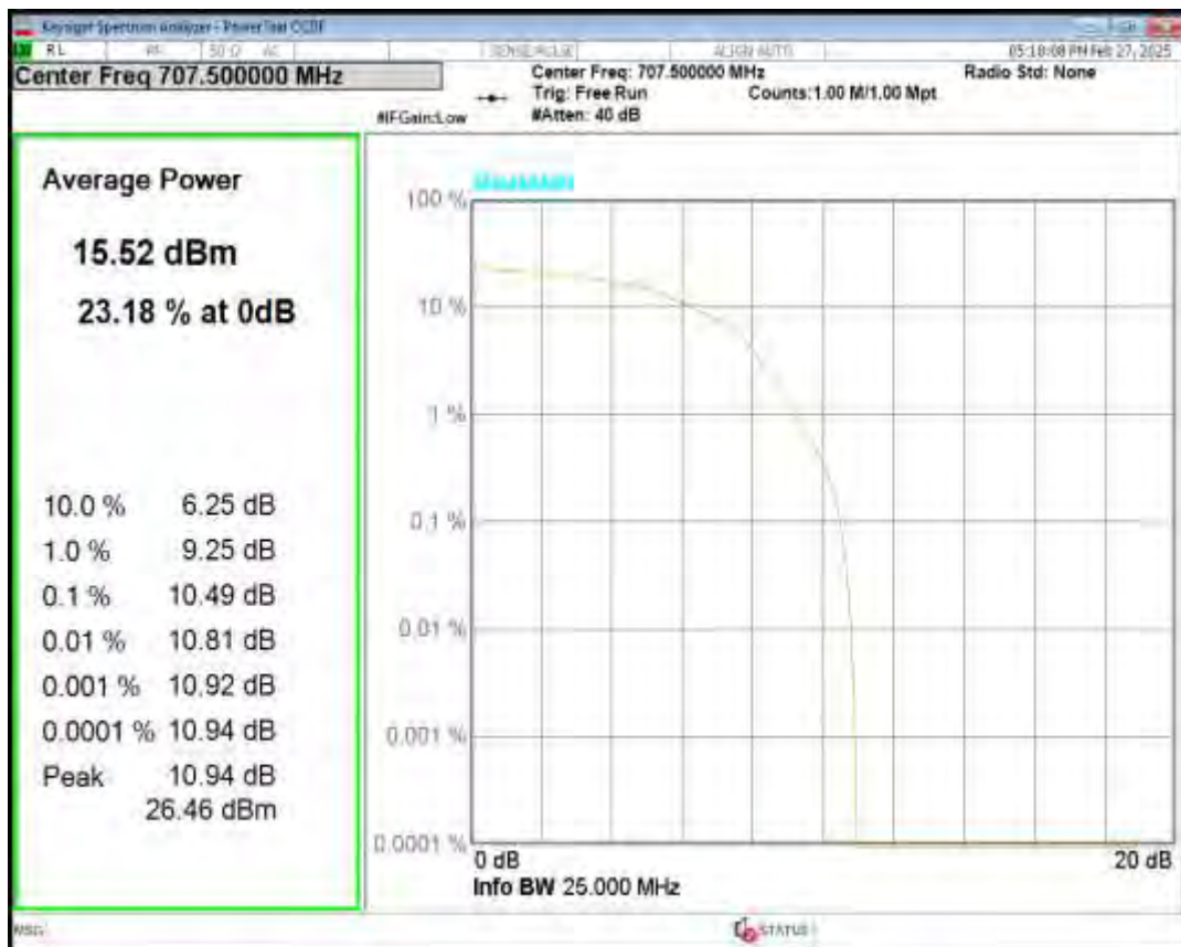
Band12 QPSK BW=5MHz Channel=23155 RB Size=6 Position=#0 NB Index=0
