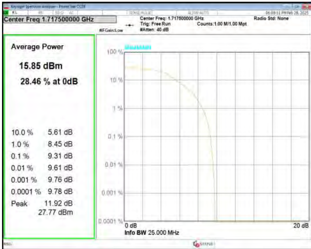
Band66 16QAM BW=15MHz Channel=132047 RB Size=5 Position=#0 NB Index=0
