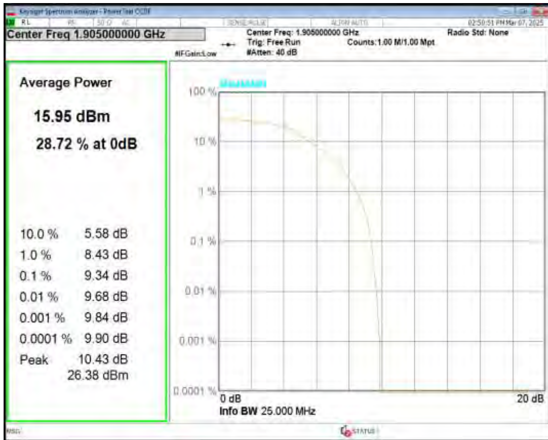
Band25 16QAM BW=20MHz Channel=26590 RB Size=5 Position=#0 NB Index=0
