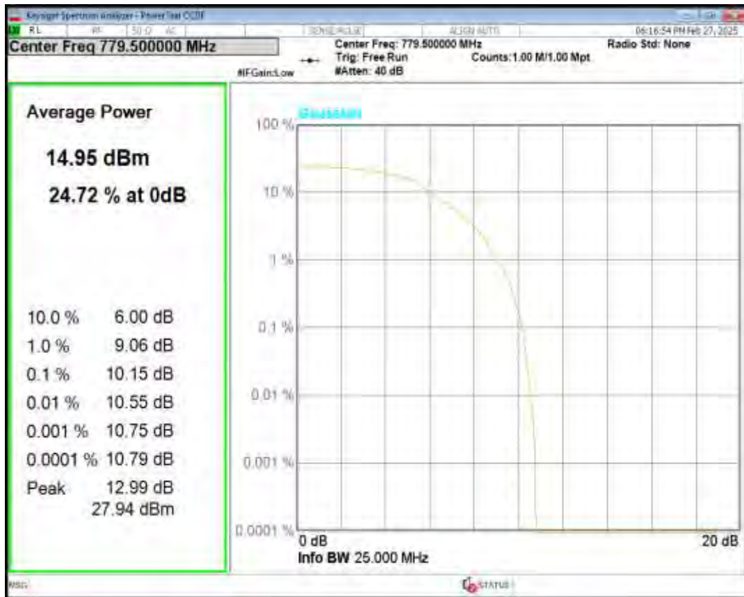
Band13 16QAM BW=5MHz Channel=23205 RB Size=5 Position=#0 NB Index=0
