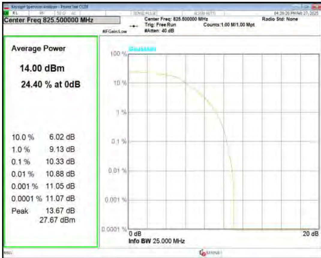
Band5 16QAM BW=3MHz Channel=20415 RB Size=5 Position=#0 NB Index=0
