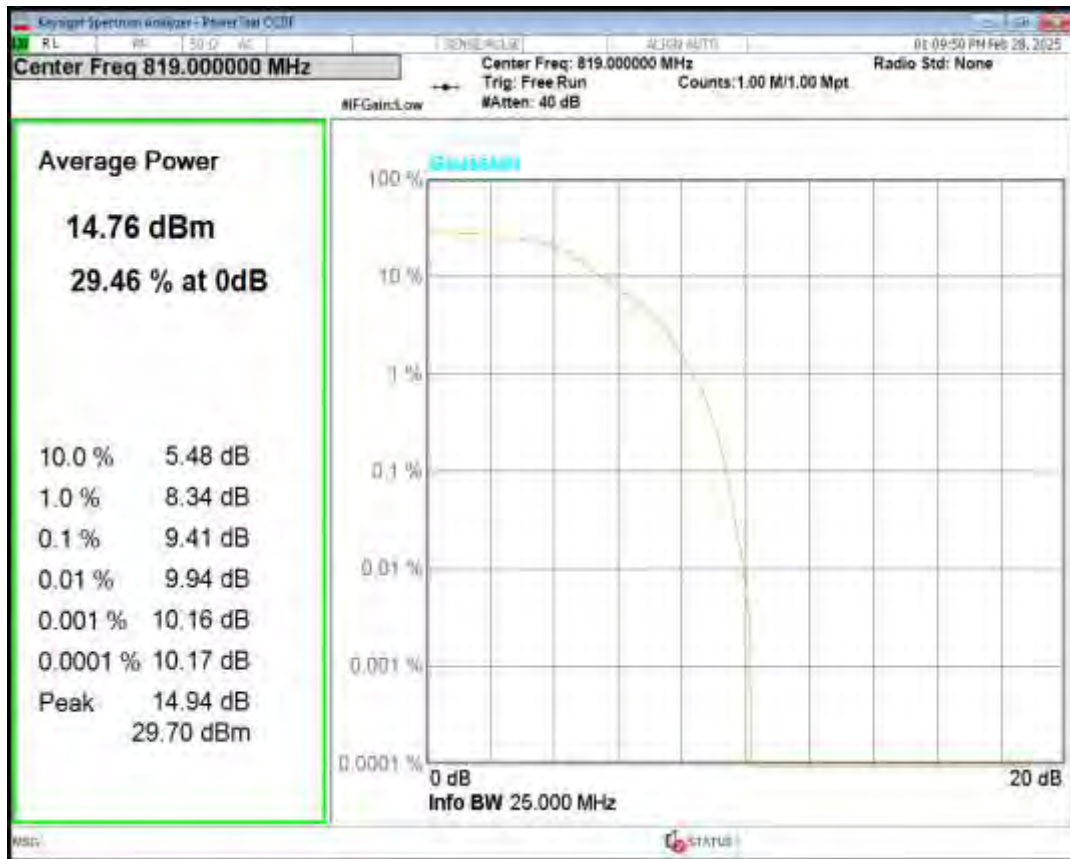
Band26(814-824) 16QAM BW=1.4MHz Channel=26740 RB Size=5 Position=#0 NB Index=0
