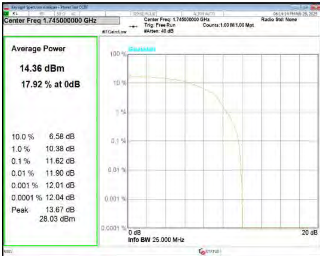
Band66 QPSK BW=20MHz Channel=132572 RB Size=6 Position=#0 NB Index=0
