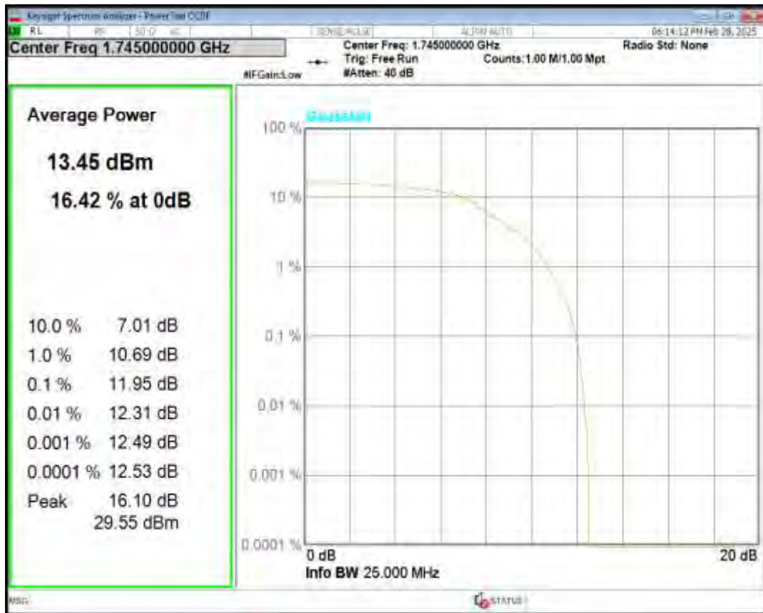
Band66 16QAM BW=20MHz Channel=132322 RB Size=5 Position=#0 NB Index=0
