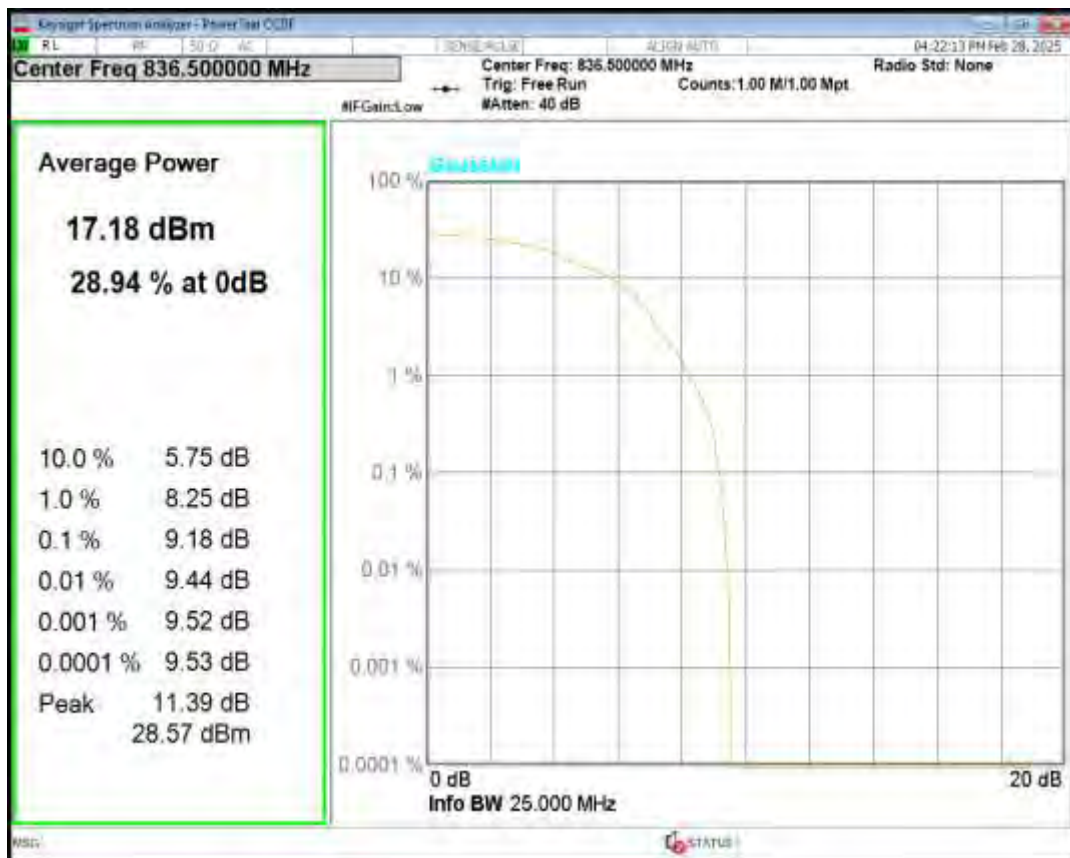
Band26(824-849) QPSK BW=10MHz Channel=26990 RB Size=6 Position=#0 NB Index=0
