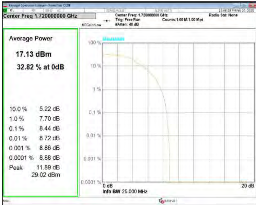
Band4 16QAM BW=20MHz Channel=20050 RB Size=5 Position=#0 NB Index=0
