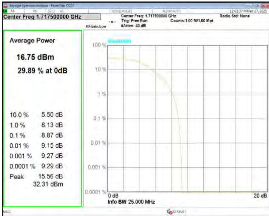
Band4 16QAM BW=15MHz Channel=20025 RB Size=5 Position=#0 NB Index=0
