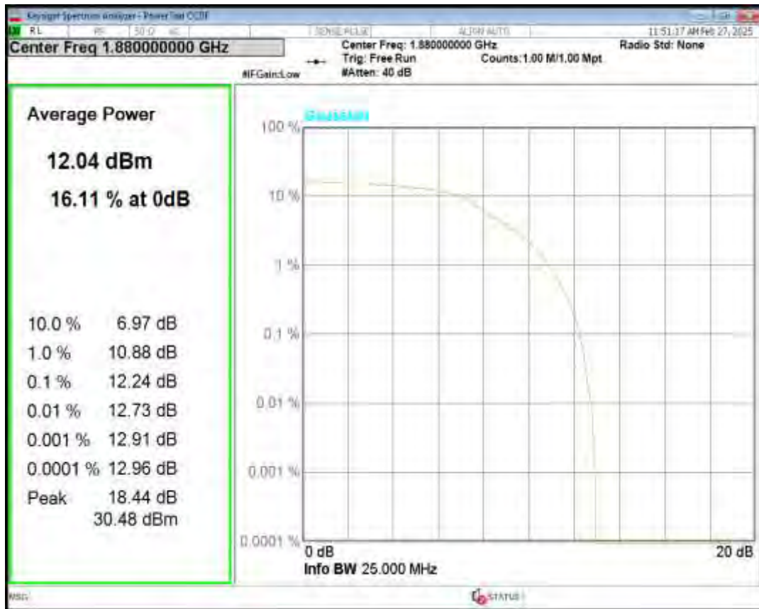
Band2 16QAM BW=3MHz Channel=18900 RB Size=5 Position=#0 NB Index=0
