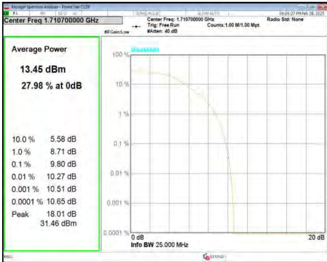
Band66 16QAM BW=1.4MHz Channel=131979 RB Size=5 Position=#0 NB Index=0
