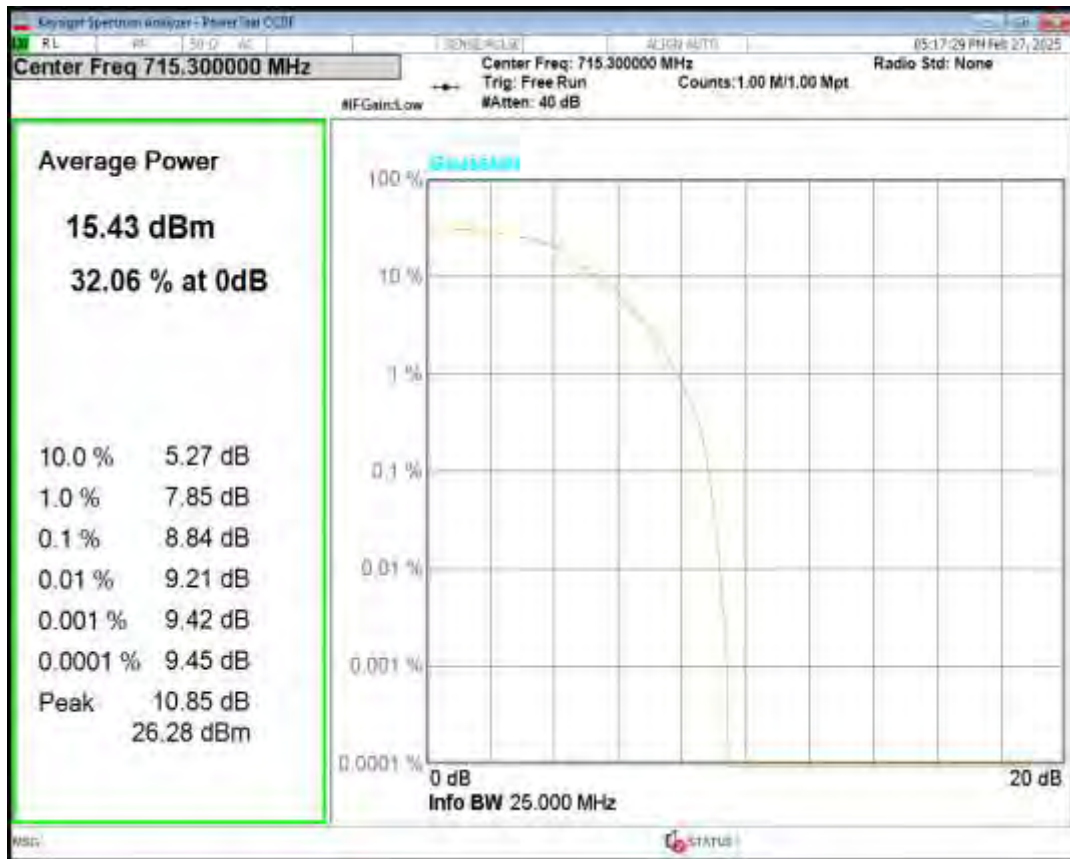
Band12 16QAM BW=1.4MHz Channel=23173 RB Size=5 Position=#0 NB Index=0
