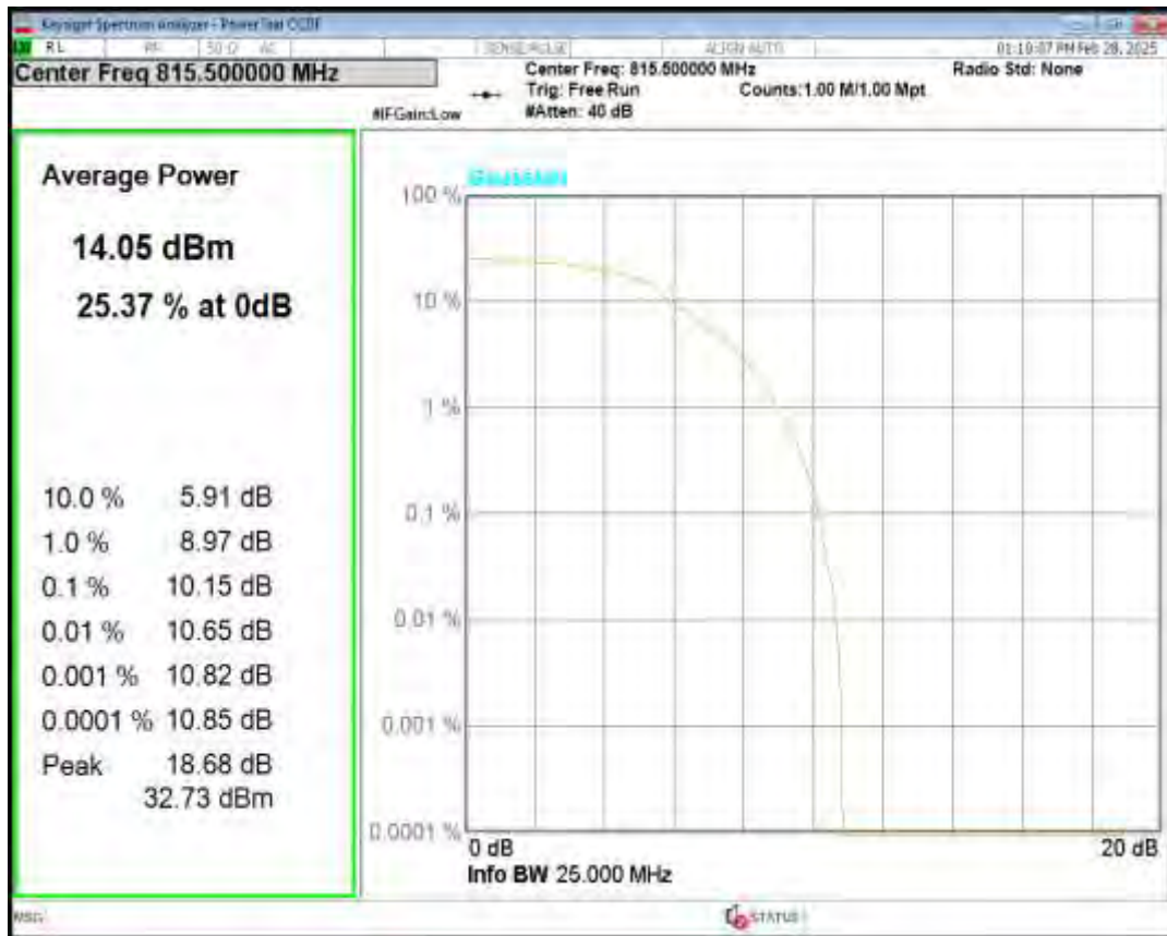
Band26(814-824) 16QAM BW=3MHz Channel=26705 RB Size=5 Position=#0 NB Index=0
