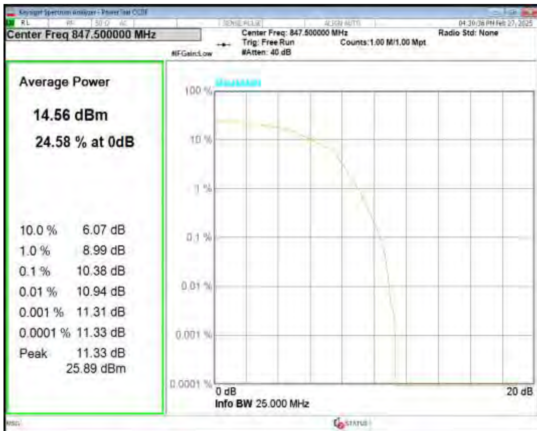
Band5 QPSK BW=5MHz Channel=20425 RB Size=6 Position=#0 NB Index=0
