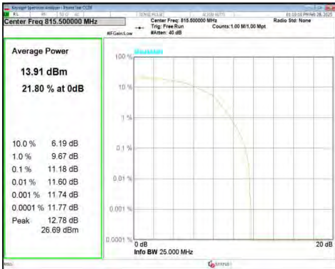
Band26(814-824) QPSK BW=3MHz Channel=26740 RB Size=6 Position=#0 NB Index=0
