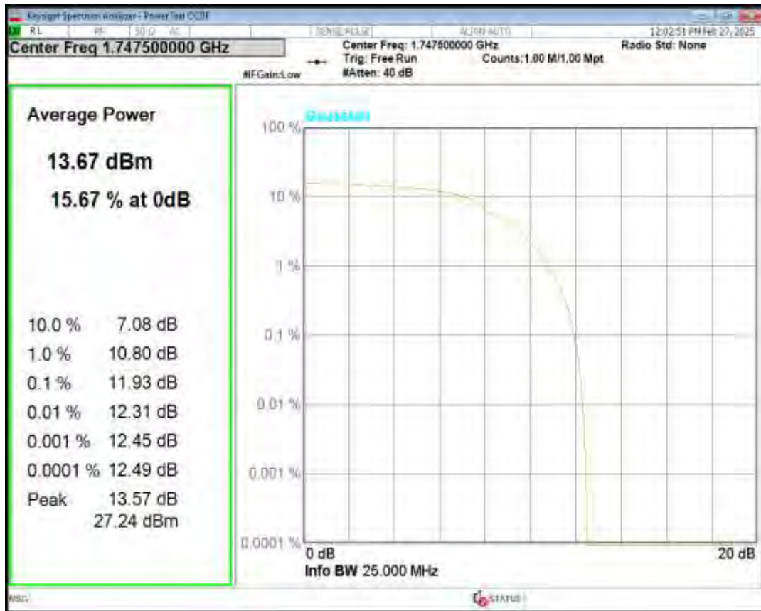
Band4 16QAM BW=15MHz Channel=20325 RB Size=5 Position=#0 NB Index=0
