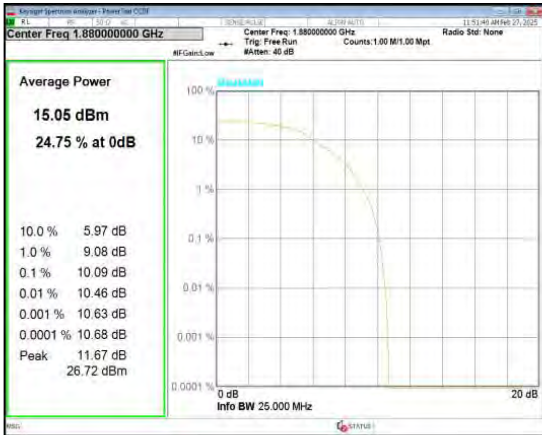
Band2 16QAM BW=5MHz Channel=18900 RB Size=5 Position=#0 NB Index=0
