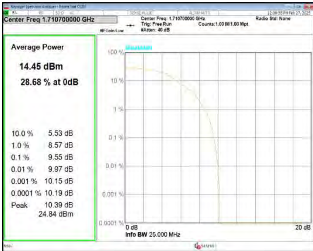
Band4 16QAM BW=1.4MHz Channel=19957 RB Size=5 Position=#0 NB Index=0
