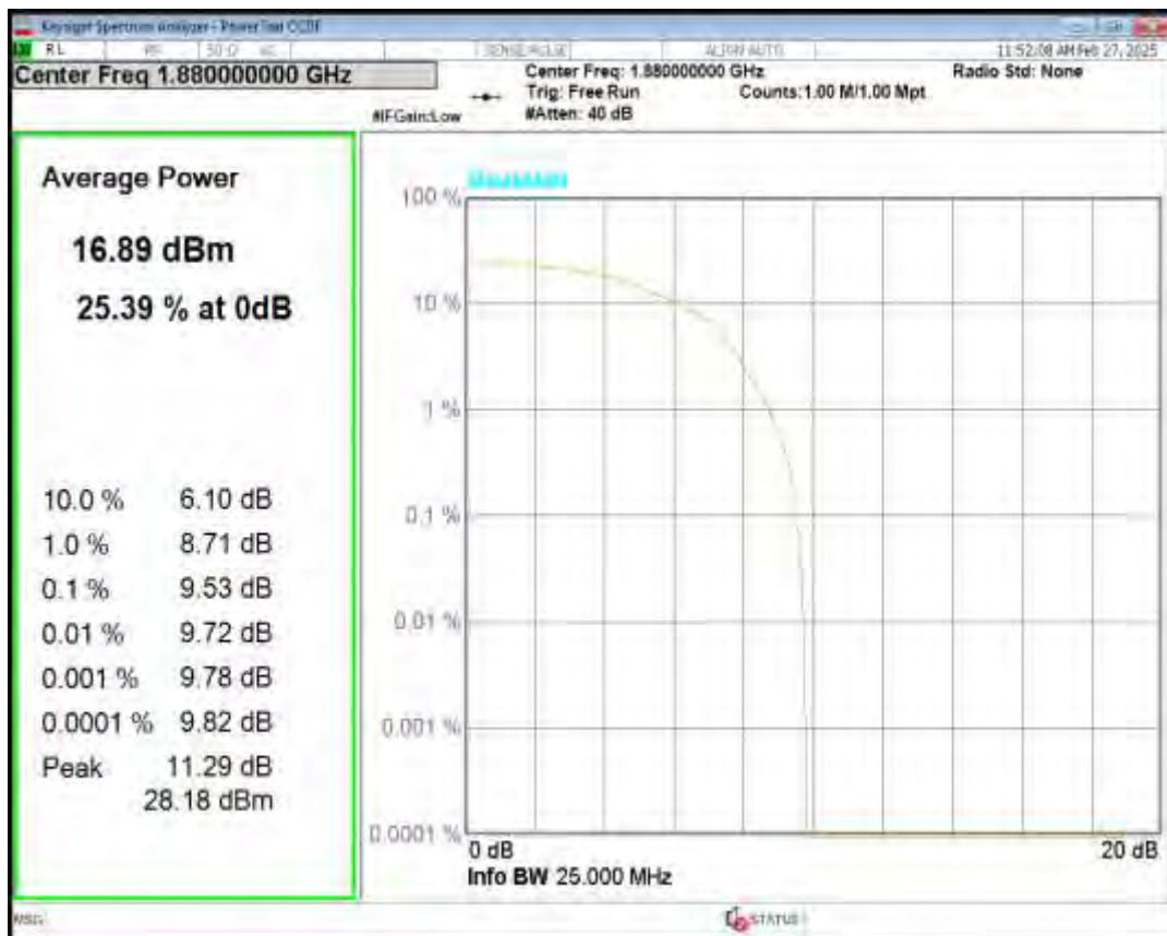
Band2 QPSK BW=10MHz Channel=19150 RB Size=6 Position=#0 NB Index=0
