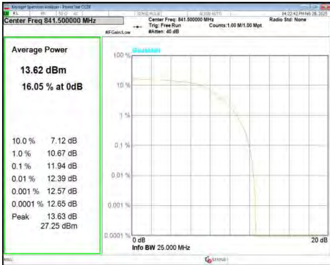
Band26(824-849) 16QAM BW=15MHz Channel=26965 RB Size=5 Position=#0 NB Index=0
