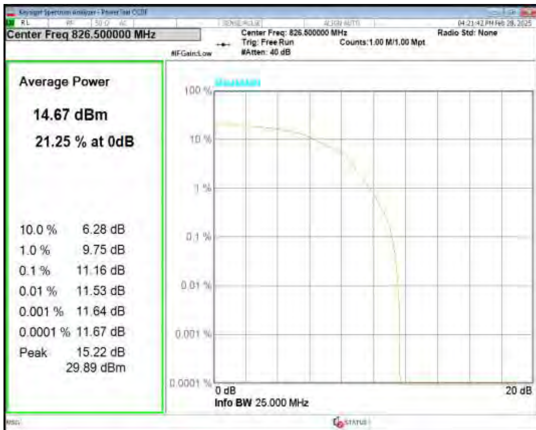
Band26(824-849) QPSK BW=5MHz Channel=26915 RB Size=6 Position=#0 NB Index=0
