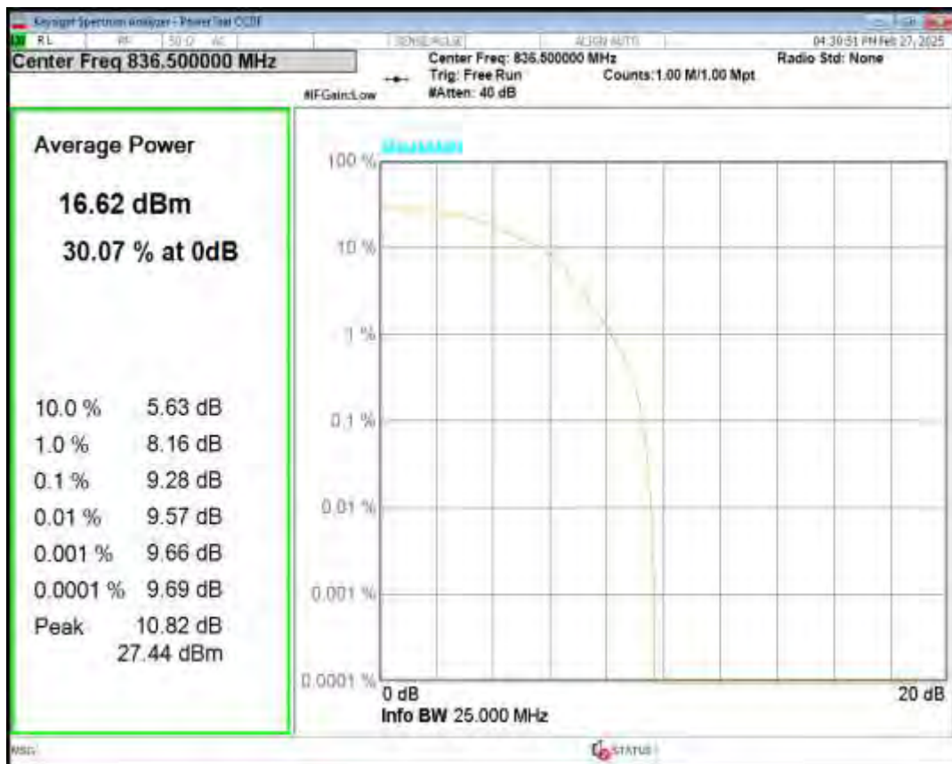
Band5 QPSK BW=5MHz Channel=20625 RB Size=6 Position=#0 NB Index=0
