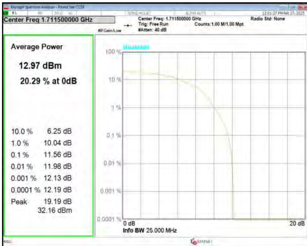
Band4 QPSK BW=3MHz Channel=20175 RB Size=6 Position=#0 NB Index=0
