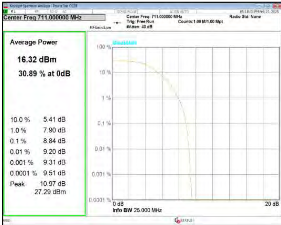
Band12 16QAM BW=10MHz Channel=23130 RB Size=5 Position=#0 NB Index=0
