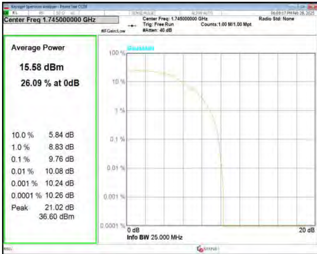
Band66 16QAM BW=15MHz Channel=132322 RB Size=5 Position=#0 NB Index=0
