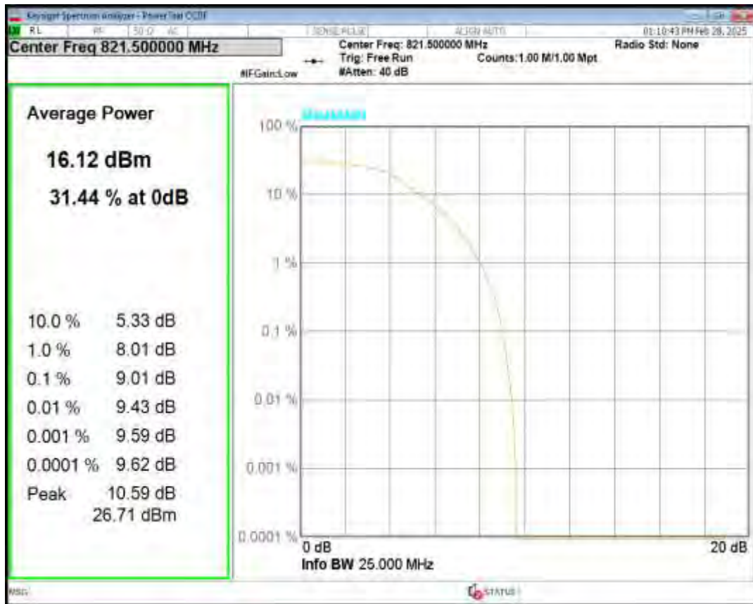
Band26(814-824) 16QAM BW=5MHz Channel=26765 RB Size=5 Position=#0 NB Index=0
