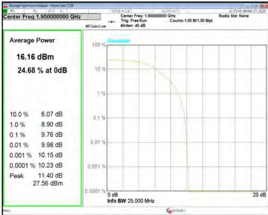
Band2 16QAM BW=20MHz Channel=19100 RB Size=5 Position=#0 NB Index=0
