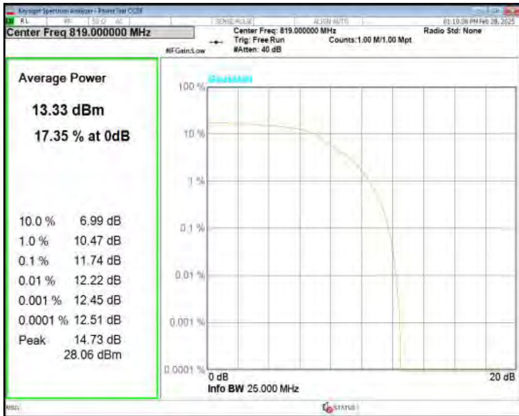
Band26(814-824) 16QAM BW=5MHz Channel=26740 RB Size=5 Position=#0 NB Index=0
