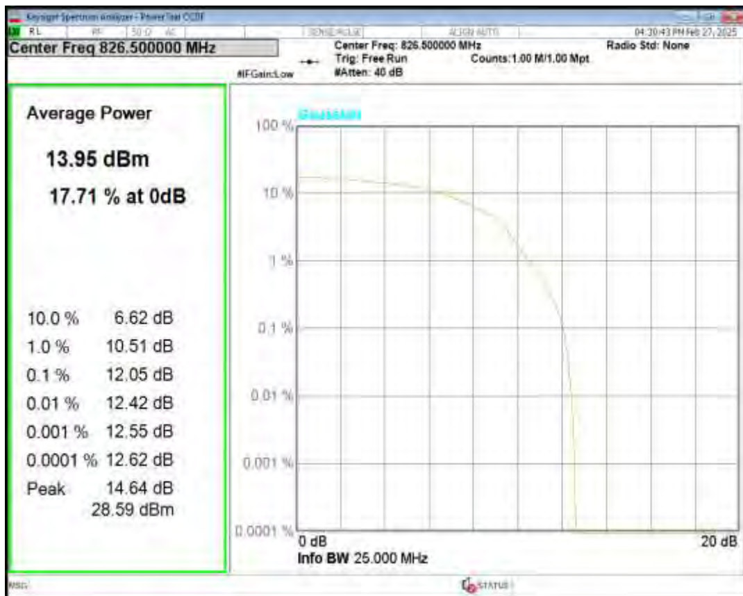
Band5 QPSK BW=5MHz Channel=20525 RB Size=6 Position=#0 NB Index=0
