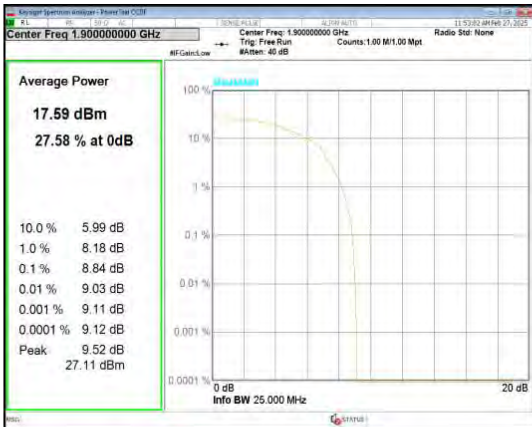
Band25 QPSK BW=1.4MHz Channel=26047 RB Size=6 Position=#0 NB Index=0
