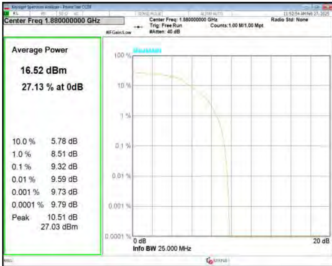
Band2 16QAM BW=20MHz Channel=18900 RB Size=5 Position=#0 NB Index=0
