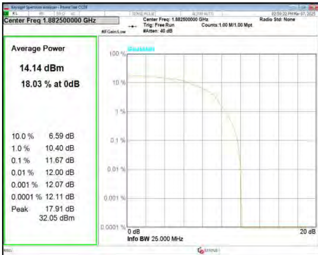
Band25 QPSK BW=15MHz Channel=26615 RB Size=6 Position=#0 NB Index=0
