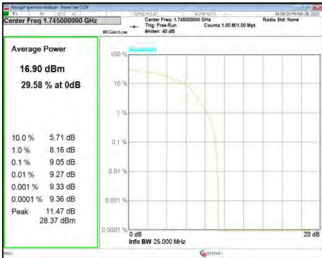
Band66 QPSK BW=15MHz Channel=132597 RB Size=6 Position=#0 NB Index=0
