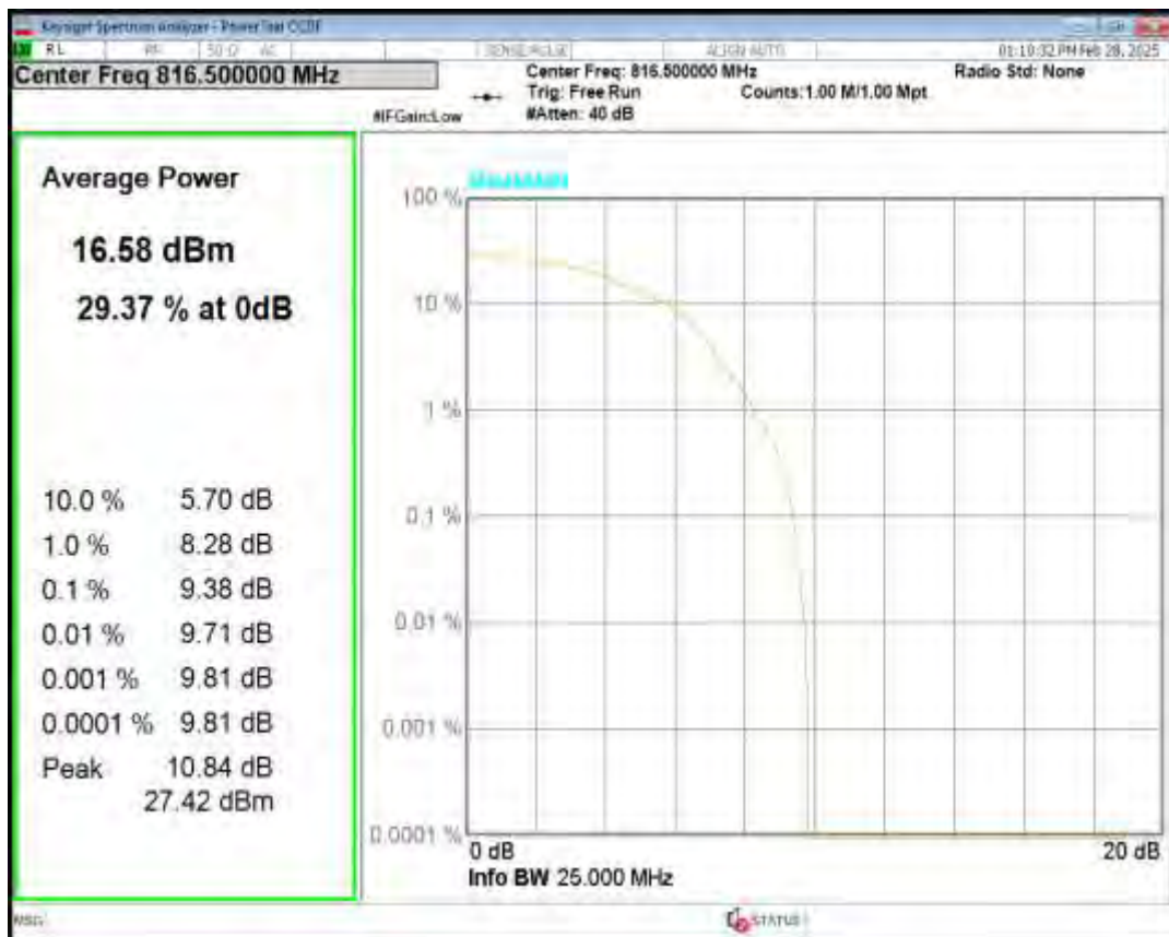
Band26(814-824) QPSK BW=5MHz Channel=26740 RB Size=6 Position=#0 NB Index=0
