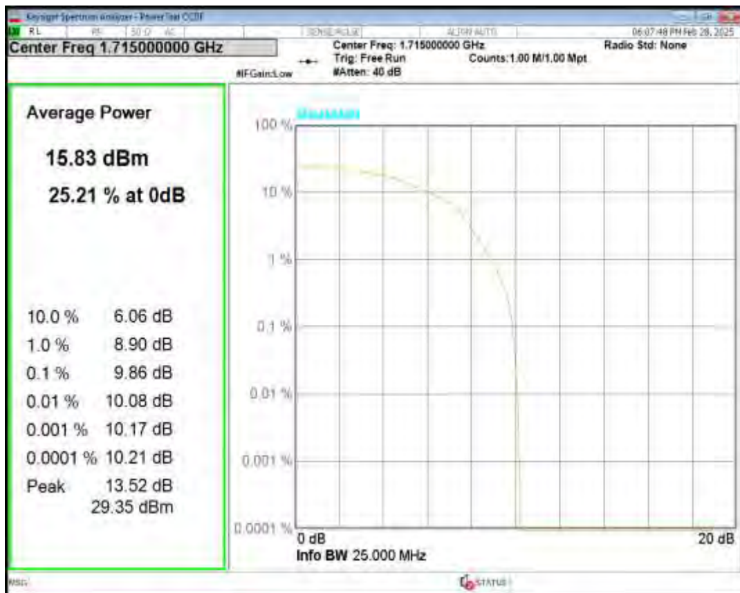
Band66 QPSK BW=10MHz Channel=132322 RB Size=6 Position=#0 NB Index=0
