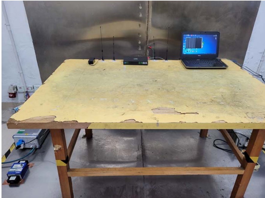
Conducted Emissions Test Setup Front View
