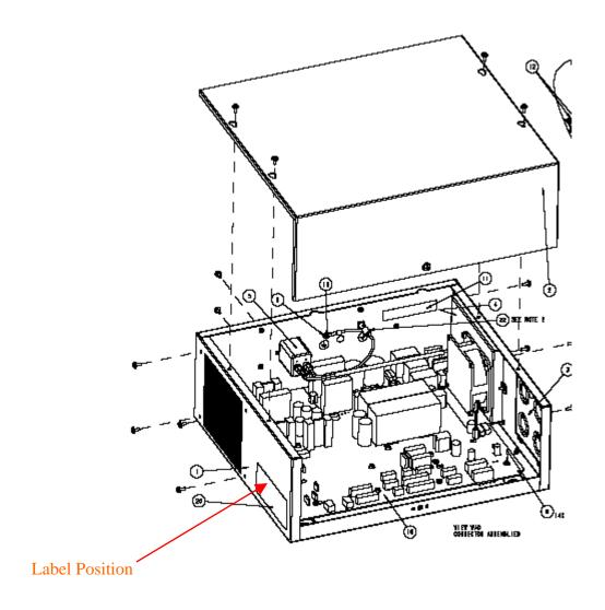
The label is a metalized polyester that is UL recognized and is permanently affixed using an L-23 adhesive.
