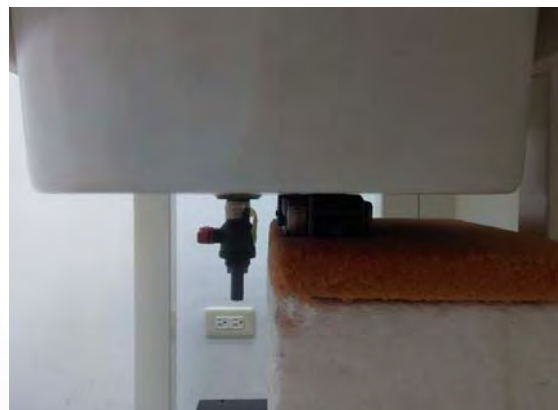
Fig.3 EUT Front side to flat phantom
