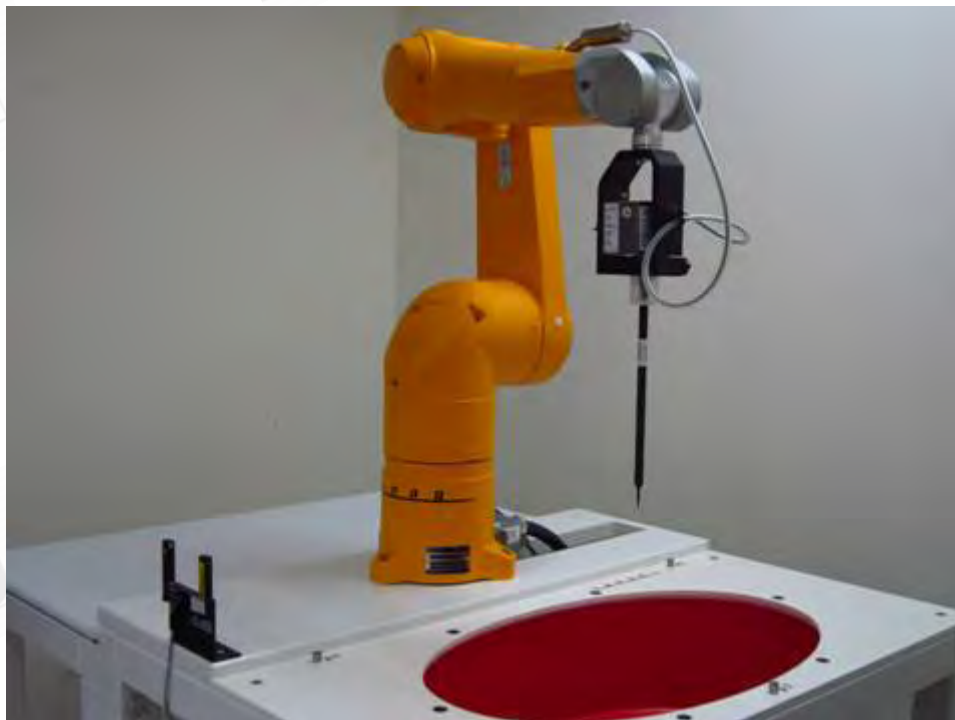
Fig.1 Photograph of the SAR measurement system
