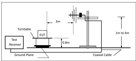
(c) For radiated emissions above 1000MHz
