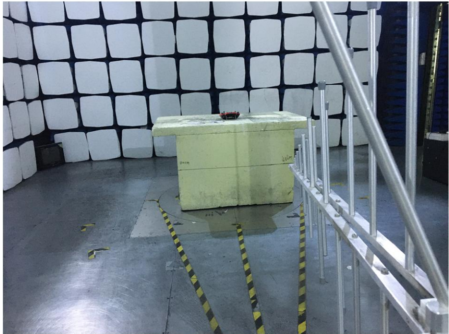
Radiation Emission Test Setup (30MHz to 1GHz)
