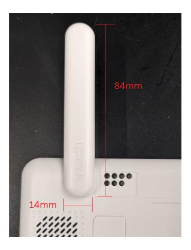
Figure 1 Physical dimension (mm)
