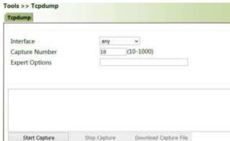
Download wireshark from the browser to open the downloaded file and analyze the messages to understand the network connection of the interface.
