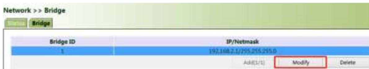
2. Modify the IP address of the bridge port or bridge members. Among the bridge members, dot11radio1 and dot11radio2 are Wi-Fi 2.4G and Wi-Fi 5G ports respectively.
