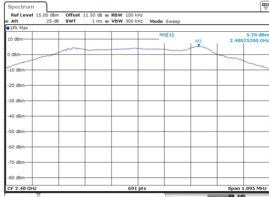
In-Band Reference Level BLE 1M_Channel 39
