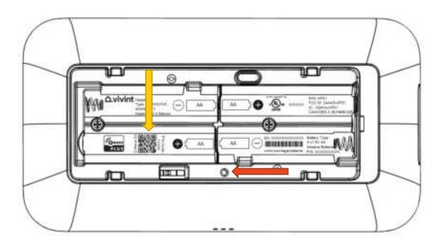
In the diagram below, the **Reset Button** used for adding/removing and factory reset pointed at by the **RED ARROW**, and the **DSK** is pointed at by the **YELLOW ARROW**.
