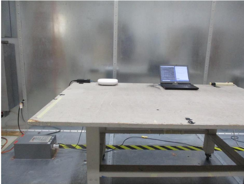
**1.10 AC Line Conducted Emission Rear View**
