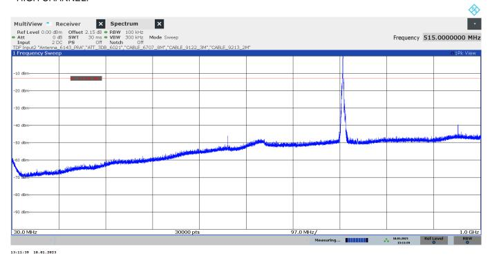
The peak above the limit is the LTE Cat-M1 Band 12 carrier frequency.
