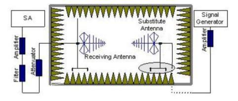
In the chamber, an substitution antenna for the frequency band of interest is placed at the
