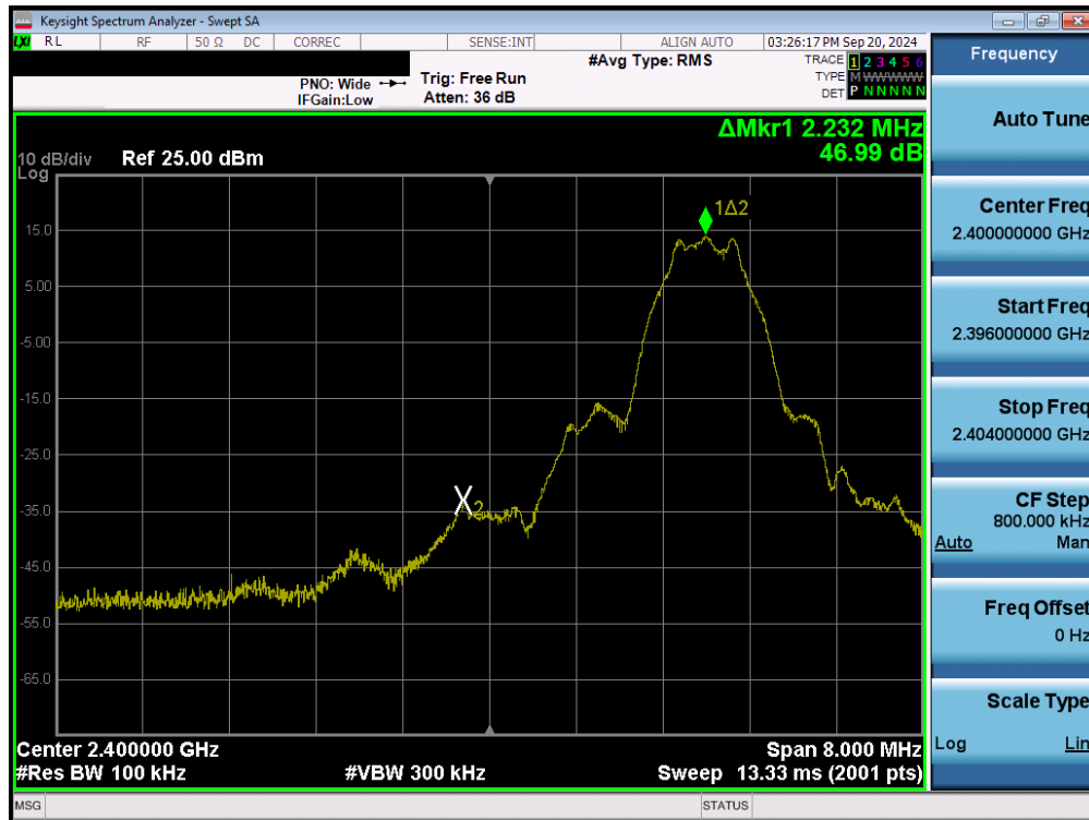
Plot 7-127. Band Edge Plot (Bluetooth (LE), 1Mbps – Ch. 37) – Dual Ant 1
