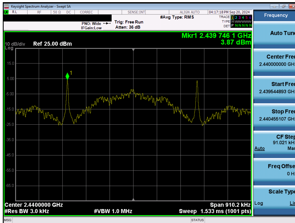
Plot 7-88. Power Spectral Density Plot (Bluetooth (LE), 125kbps – Ch. 17) – Ant 2
