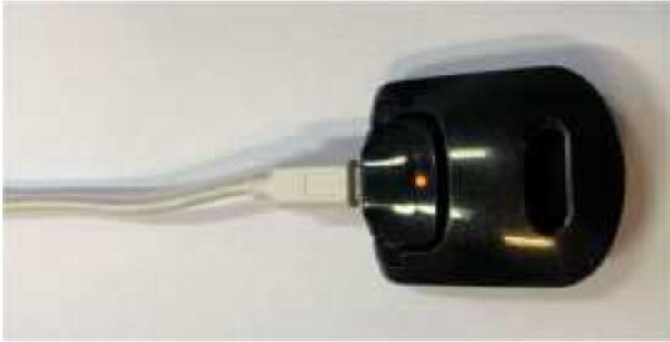
2. Check that the LED goes green to indicate that the Charger is fully charged (this could take up to 2 hours).
