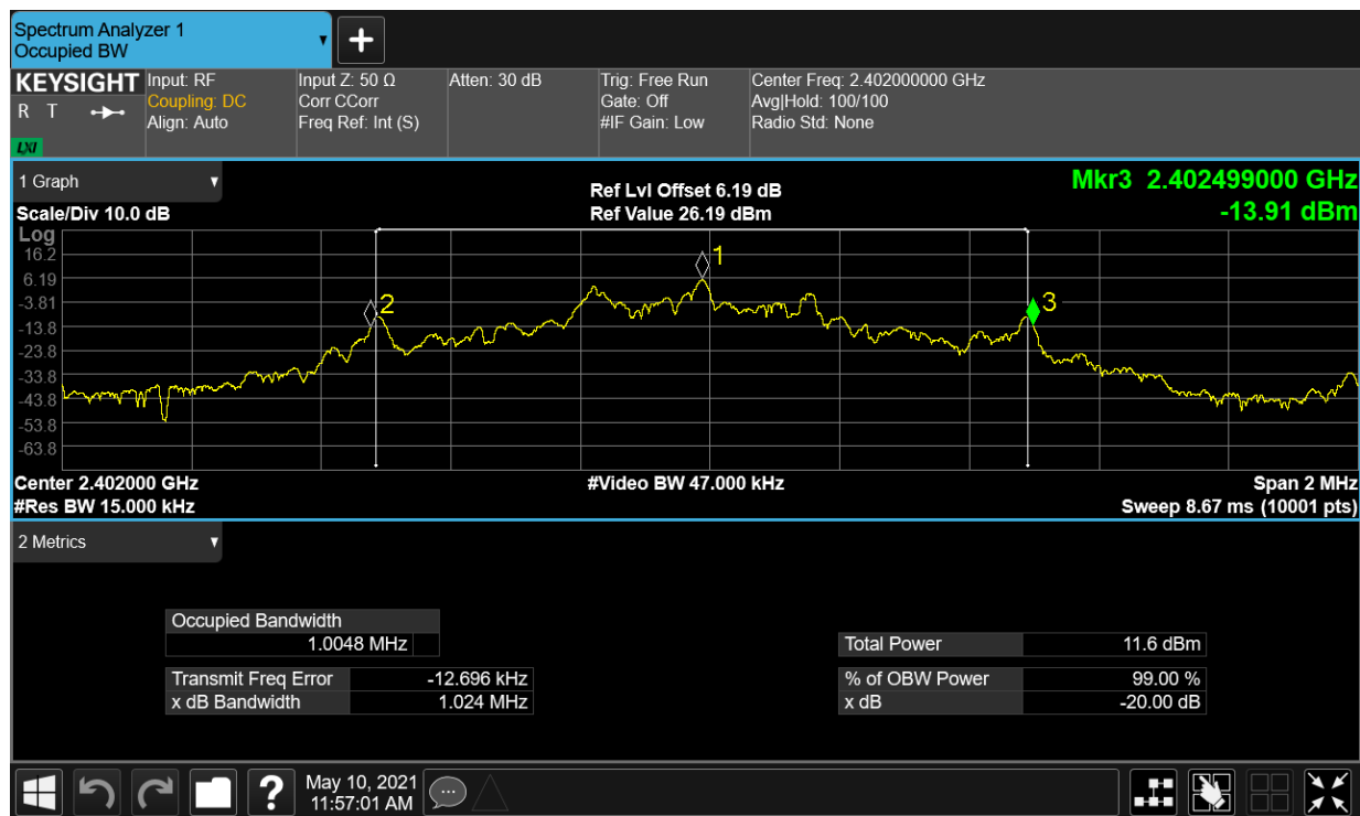
-20dB Bandwidth NVNT 1-DH1 2441MHz Ant1
