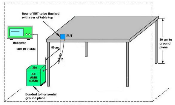
AMN = Artificial mains network (LISN) AE = Associated equipment EUT = Equipment under test
