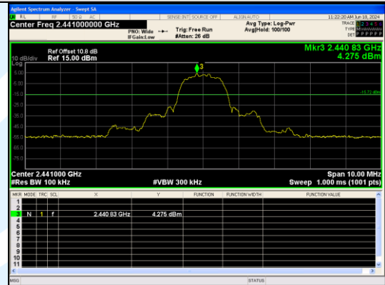
Out Of Band Emission 8DPSK_3-DH5_Channel 39
