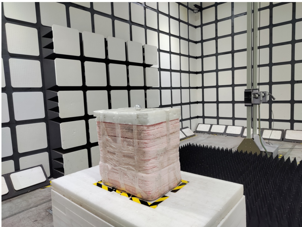
Radiated Emissions View (1-18 GHz)
