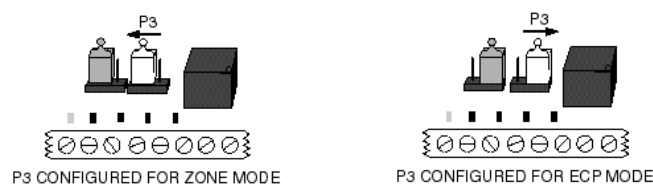
Figure 5. K3852 P3 Jumper Configuration
