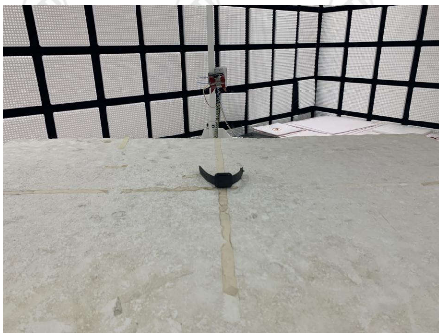
Radiated spurious emission Test Setup-2(Above 1GHz)
