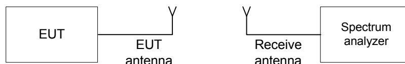
Figure 7.7.1 Band edge emission test setup
