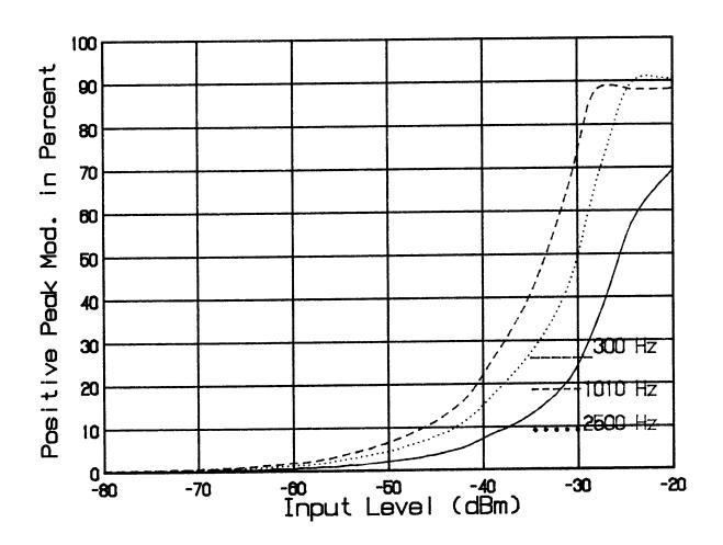
Percent modulation as a function of input level at microphone jack in dBm for 300 Hz, 1010 Hz, and 2500 Hz tones.
