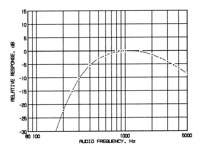
TRANSMITTER FREQUENCY RESPONSE MODEL HH37ST (Normal)
