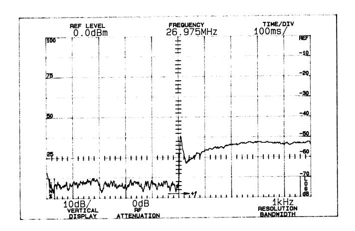
Measurement Conditions: 16 dB over 50% modulation level at 1820 Hz with 2500 Hz tone, upper fourth order sideband; horizontal scale 100 ms/div.
