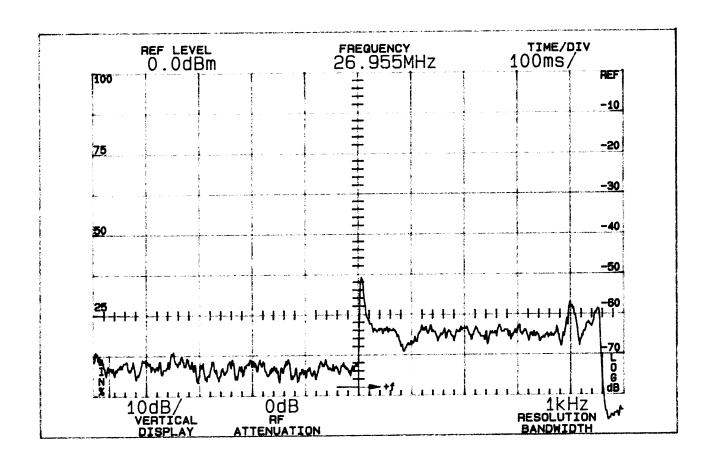
Measurement Conditions: 16 dB over 50% modulation level at 1010 Hz with 2500 Hz tone, lower fourth order sideband; horizontal scale 100 ms/div.
