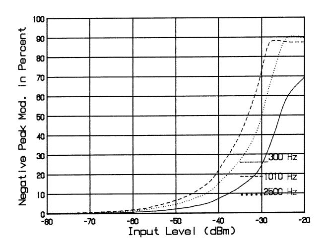
Percent modulation as a function of input level at microphone jack in dBm for 300 Hz, 1010 Hz, and 2500 Hz tones.
