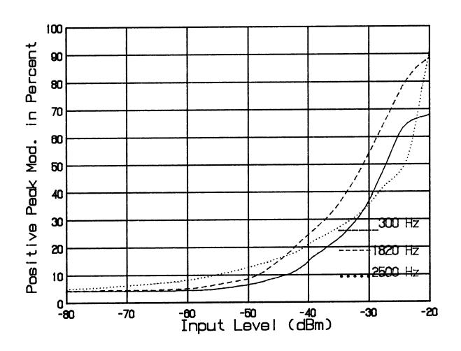
Percent modulation as a function of input level at microphone jack in dBm for 300 Hz, 1820 Hz, and 2500 Hz tones.
