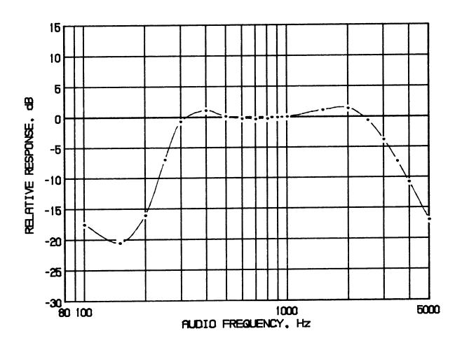
TRANSMITTER FREQUENCY RESPONSE MODEL HH37ST (ST Mode)
