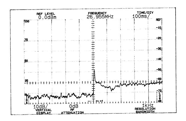
Measurement Conditions: 16 dB over 50% modulation level at 1820 Hz with 2500 Hz tone, lower fourth order sideband; horizontal scale 100 ms/div.
