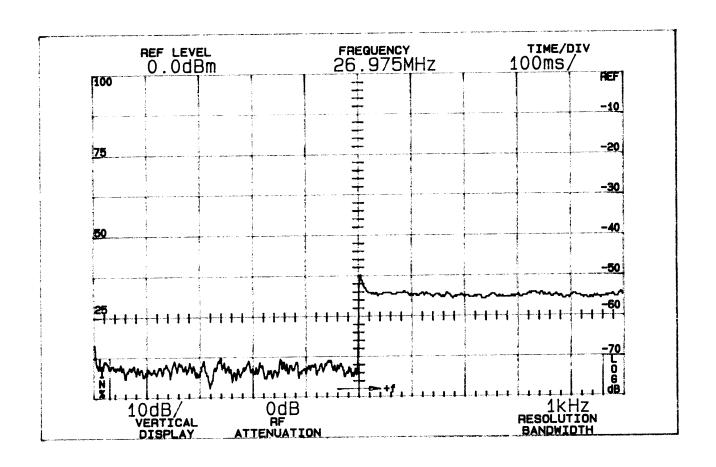
Measurement Conditions: 16 dB over 50% modulation level at 1010 Hz with 2500 Hz tone, upper fourth order sideband; horizontal scale 100 ms/div.
