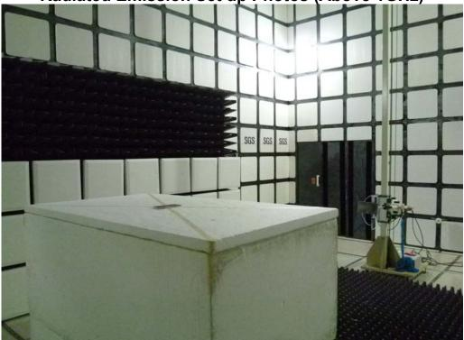
Radiated Emission Set up Photos (Front View)
