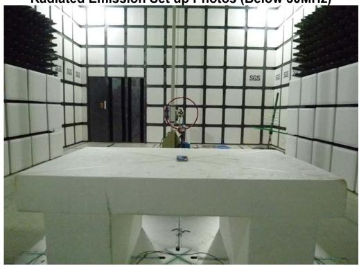
Radiated Emission Set up Photos (Below 1GHz)
