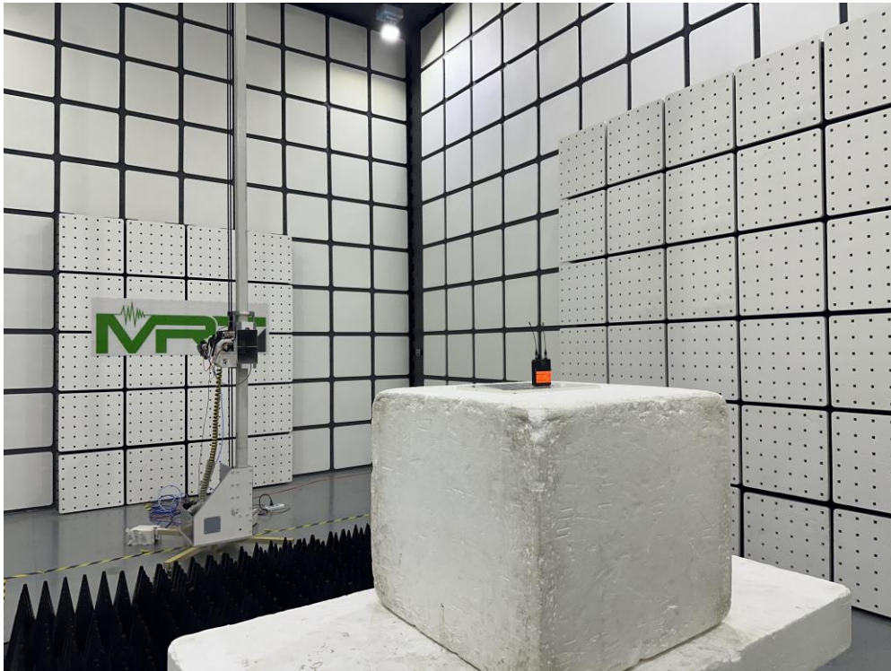
Description: RF Conducted Test Setup
