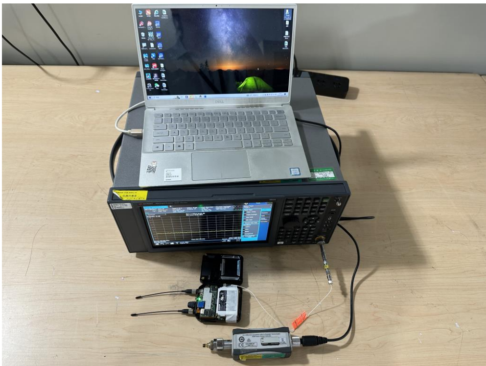
Description: RF Conducted Test Setup
