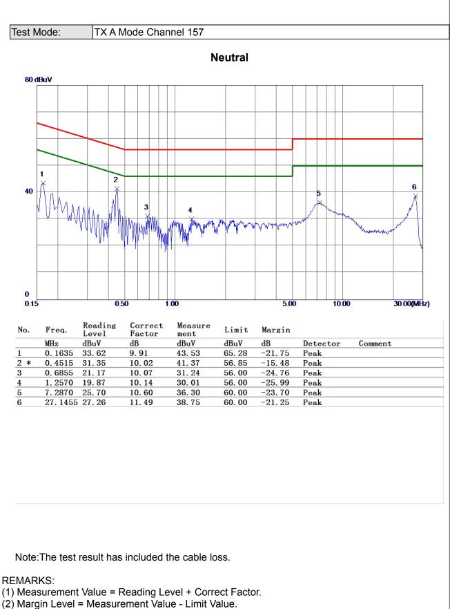
(3) The test result has included the cable loss.
