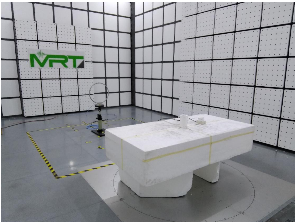
Description: Radiated Emission Test Setup for 9kHz~30MHz
