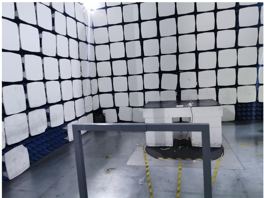
Radiation Emission Test Setup (Below 30MHz)
