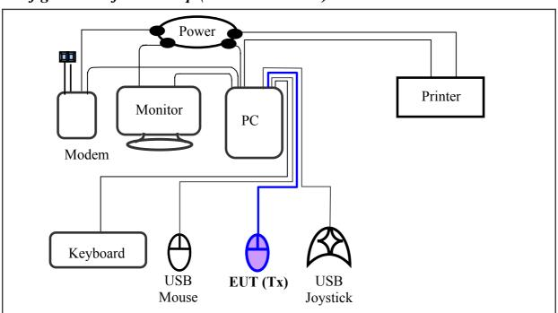
Configuration of Test Setup (Test mode: "#3")
