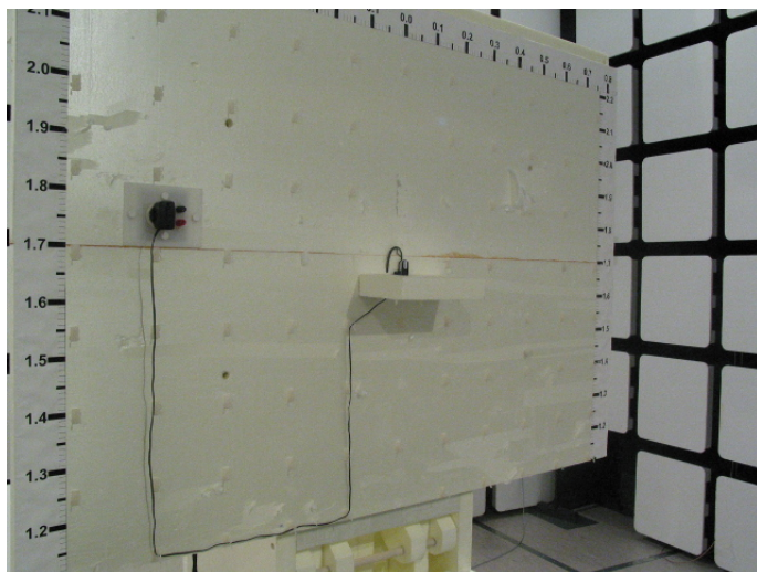
Picture 1 Spurious radiated emission measurement Bluetooth TX
