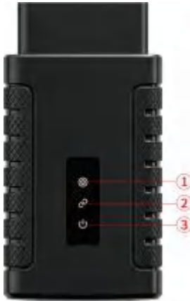
Figure 2-4 Front View of VCI dongle
