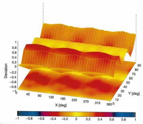
Probe isotropy for  $E_{tot}$ : probe rotated  $\phi = 0^{\circ}$  to 360°, tilted from field propagation direction  $\vec{k}$ Parallel to the field propagation ( $\psi=0^{\circ}-90^{\circ}$ ) at 30 GHz: deviation within  $\pm 0.29$  dB Parallel to the field propagation ( $\psi=0^{\circ}-90^{\circ}$ ) at 60 GHz: deviation within  $\pm 0.41$  dB
