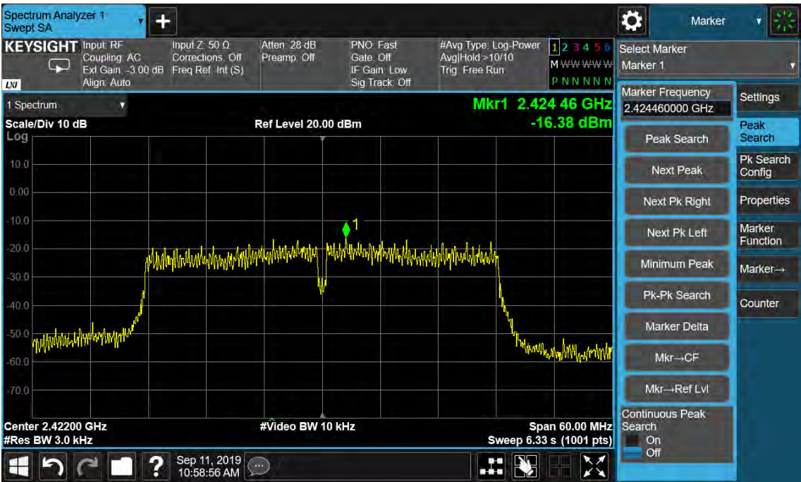
Figure 22: Power Spectral Density, 802.11n(HT40), 2422MHz
