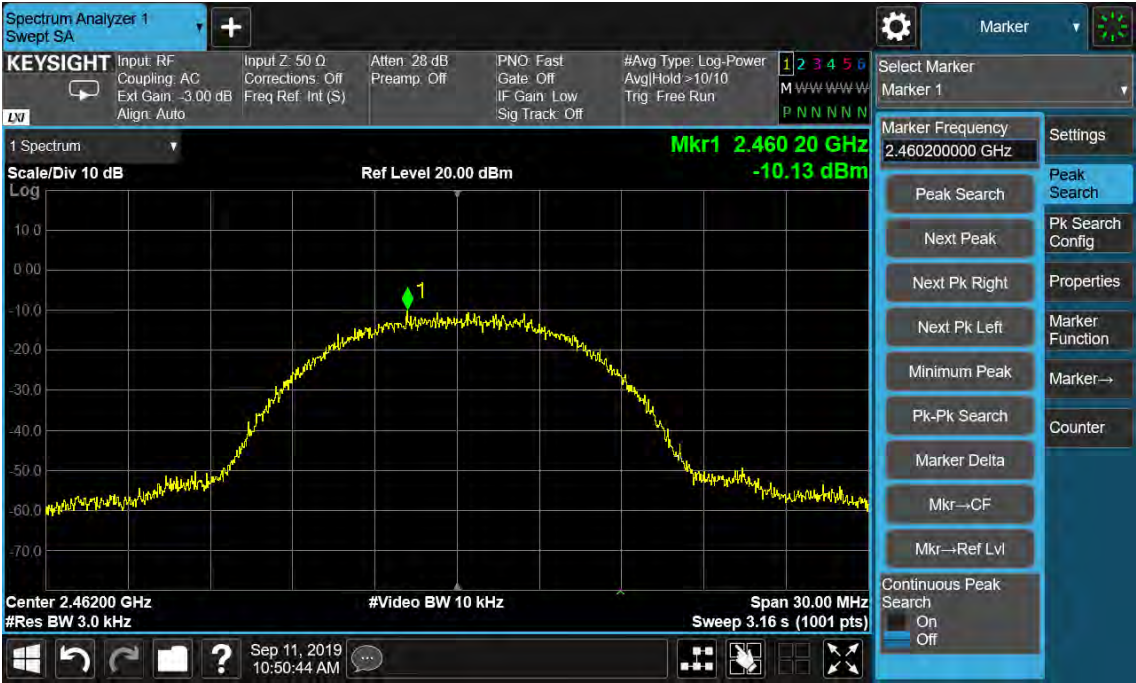
Figure 15: Power Spectral Density, 802.11b, 2462MHz
