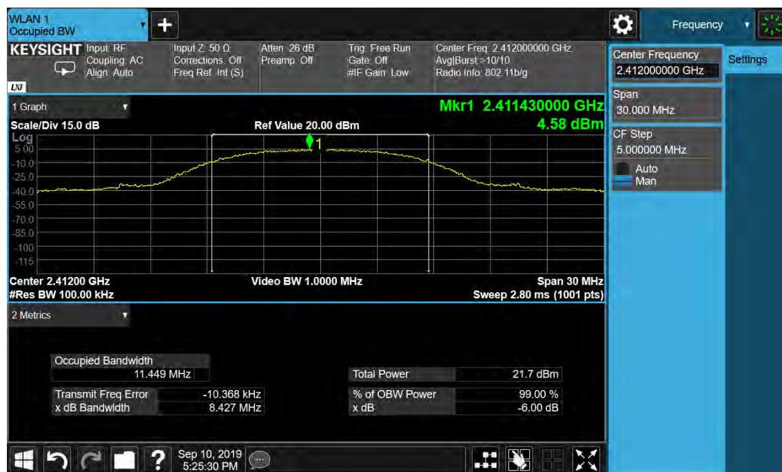
Figure 1: 6dB Bandwidth and 99% Bandwidth, 802.11b, 2412MHz
