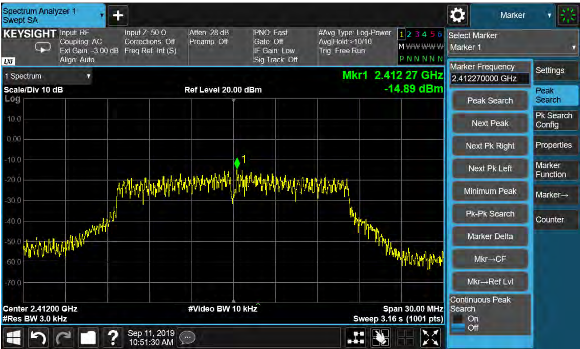
Figure 16: Power Spectral Density, 802.11g, 2412MHz
