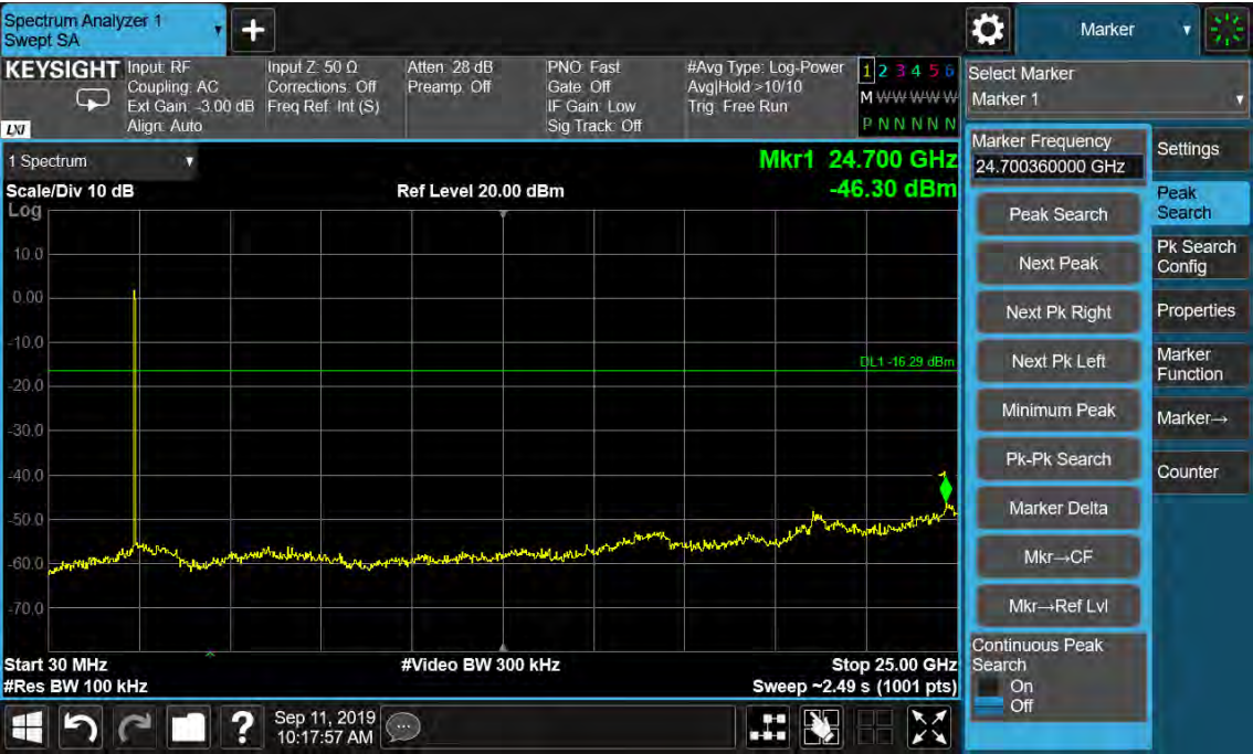
Figure 26: Conducted Spurious Emission & Authorized-band band-edge, 802.11b, 2437MHz Carrier Level
