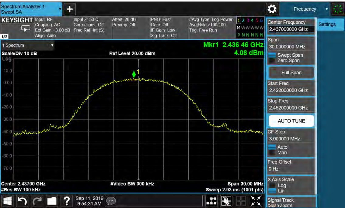
Figure 26: Conducted Spurious Emission & Authorized-band band-edge, 802.11b, 2437MHz Carrier Level
