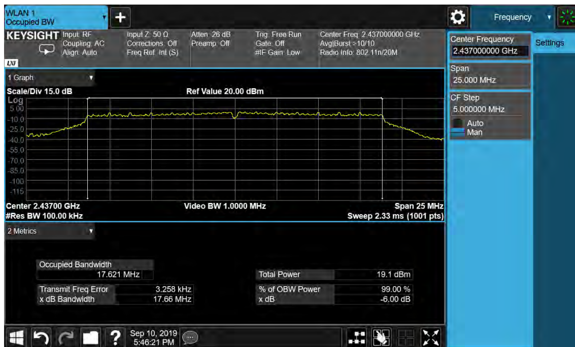
Figure 8: 6dB Bandwidth and 99% Bandwidth, 802.11n(HT20), 2437MHz
