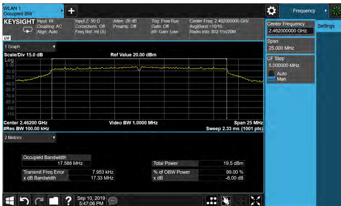
Figure 9: 6dB Bandwidth and 99% Bandwidth, 802.11n(HT20), 2462MHz
