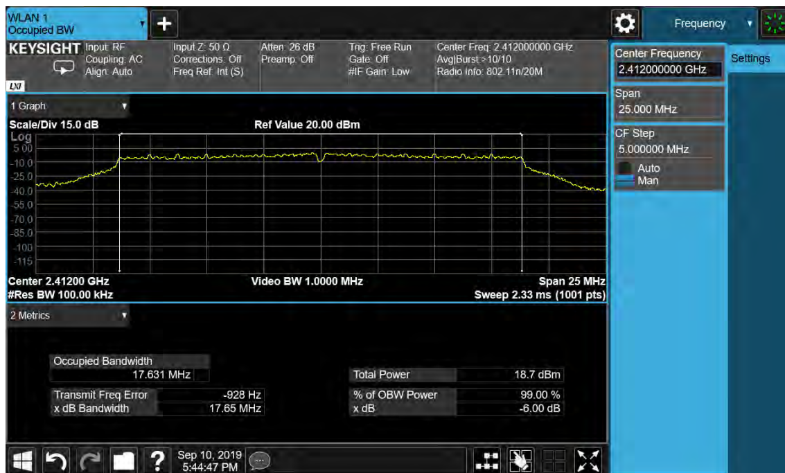
Figure 7: 6dB Bandwidth and 99% Bandwidth, 802.11n(HT20), 2412MHz
