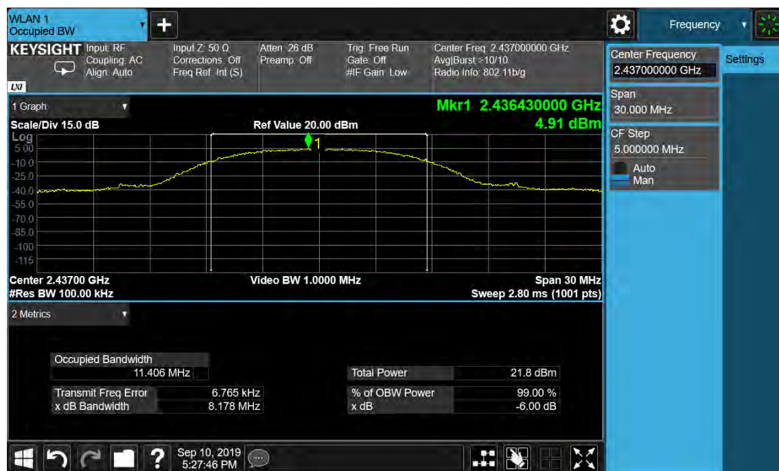
Figure 2: 6dB Bandwidth and 99% Bandwidth, 802.11b, 2437MHz
