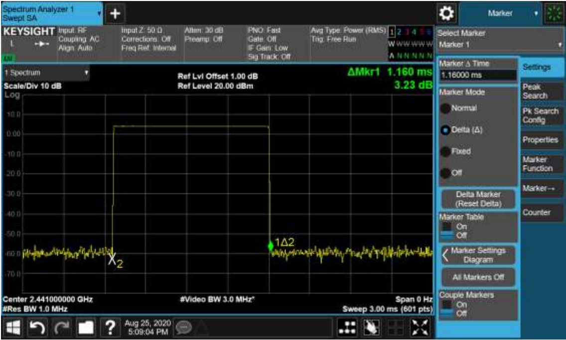
Figure 27: Time of Occupancy, 2441MHz, GFSK DH3
