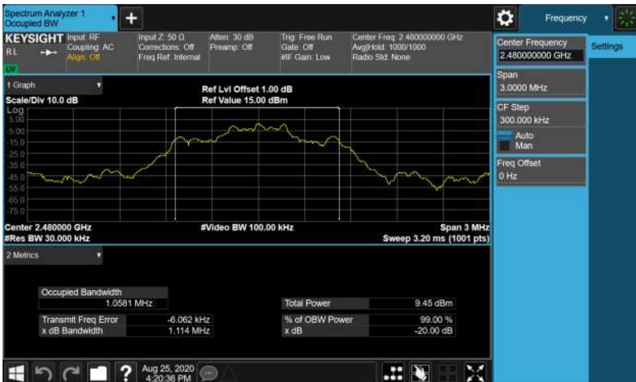
Figure 15: 20dB Bandwidth and 99% Bandwidth, 2480MHz, 8-DPSK
