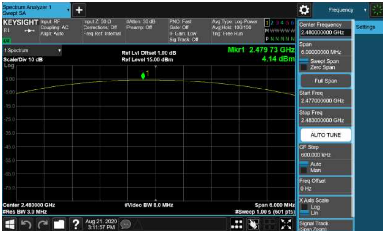
Figure 3: Maximum Conducted Output Power, 2480MHz, GFSK
