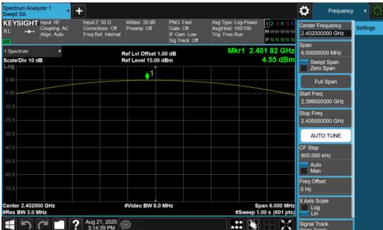
Figure 4: Maximum Conducted Output Power, 2402MHz, \pi/4 -DQPSK
