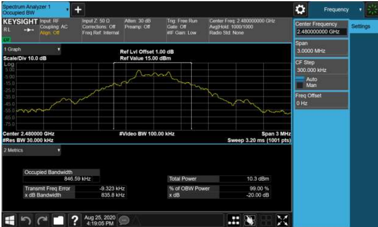
Figure 12: 20dB Bandwidth and 99% Bandwidth, 2480MHz, GFSK
