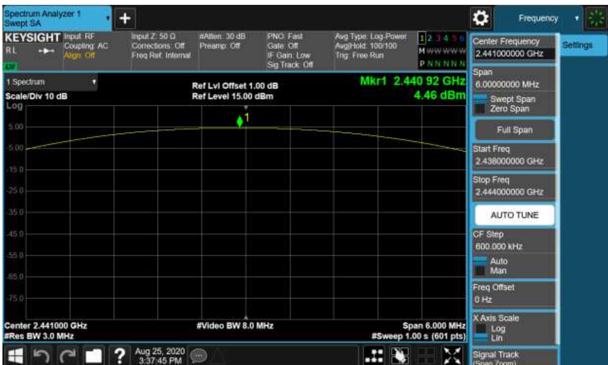
Figure 2: Maximum Conducted Output Power, 2441MHz, GFSK
