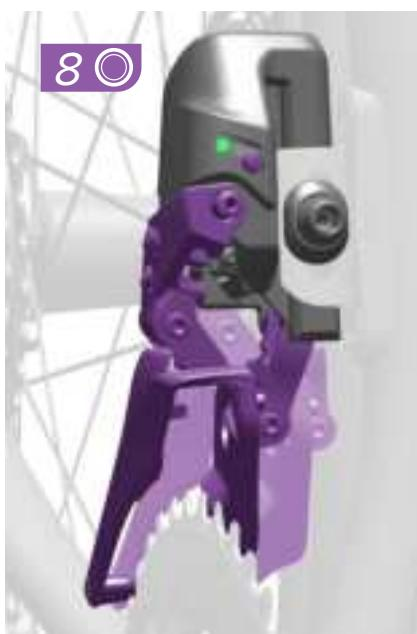
Shift the derailleur into the outward position.
