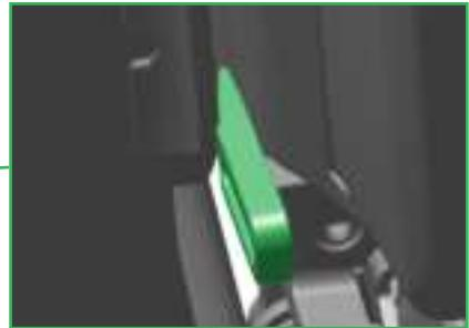
Place the flat side of each wedge against the front derailleur and slide the wedge forward until it lightly contacts the frame or braze-on. Select the wedge that best fills the gap between the frame or braze-on and the derailleur without moving the derailleur.
