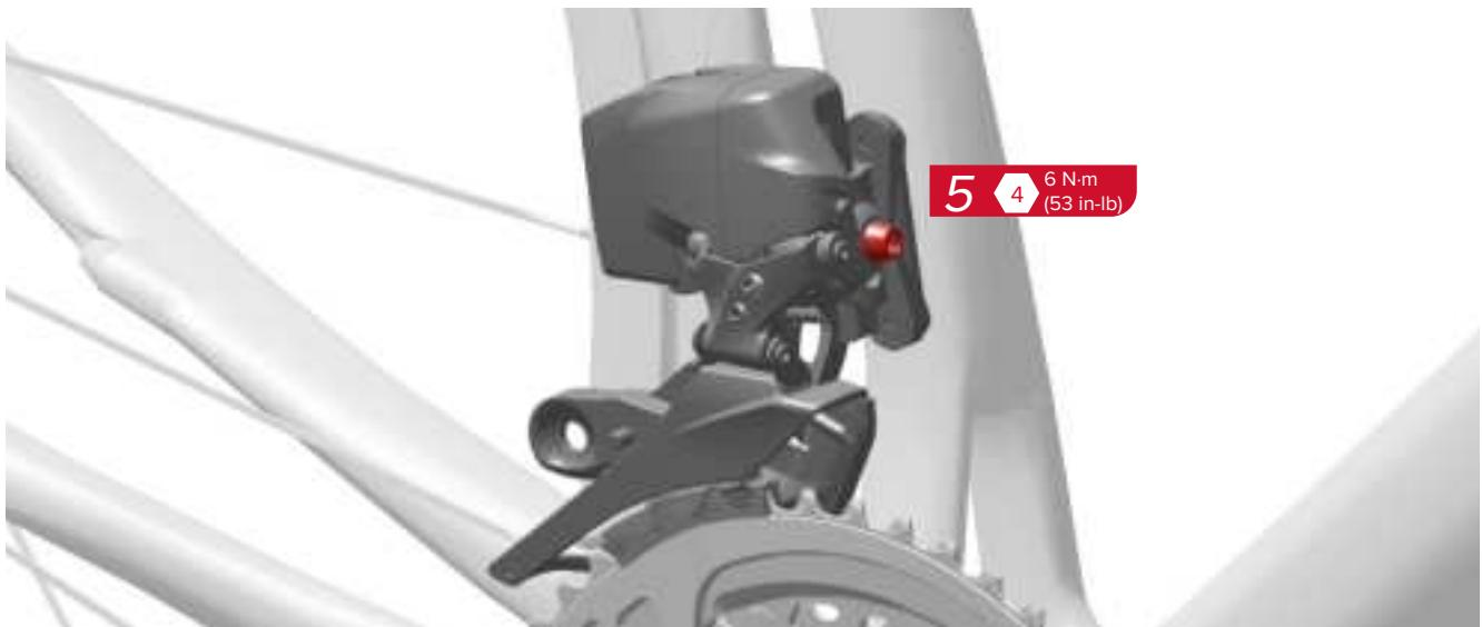
Make sure the tool is still bottomed on the chainring. While holding the tail of the derailleur cage in place, tighten the derailleur bolt. Verify the derailleur did not move during tightening.
