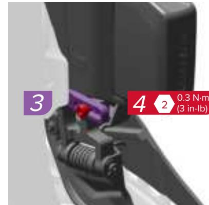
Loosely install the wedge bolt and the wedge onto the derailleur, then adjust the wedge so the tab contacts the bottom of the derailleur body.
