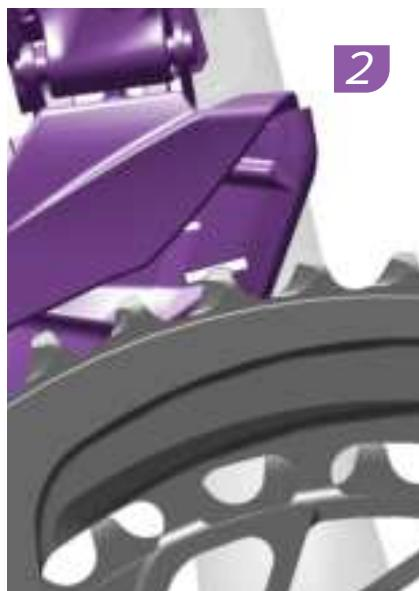
Adjust the derailleur so that the tip of the tallest chainring tooth appears within the setup line when viewed directly from the side.
