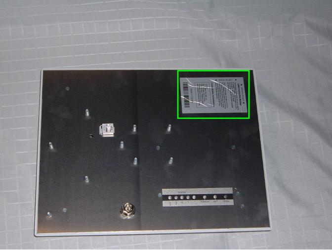
Figure 1 – External back panel, FCC Label location..
