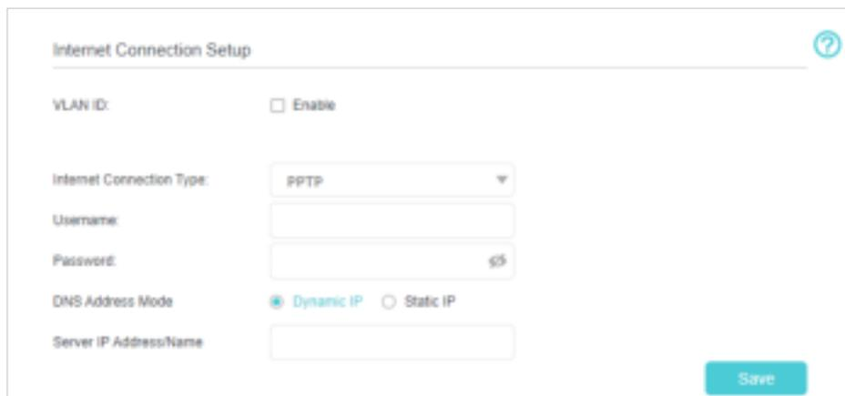
The screenshot shows the 'Internet Connection Setup' form. The 'Internet Connection Type' dropdown menu is set to 'PPTP'. The 'DNS Address Mode' section has 'Dynamic IP' selected and 'Static IP' unselected. There is an input field for 'Server IP Address/Name'. A 'Save' button is at the bottom right.
