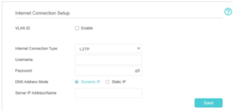
The screenshot shows the 'Internet Connection Setup' form. The 'Internet Connection Type' dropdown menu is set to 'L2TP'. Below the 'Password' field, there are radio buttons for 'DNS Address Mode', with 'Dynamic IP' selected and 'Static IP' unselected. There is also an input field for 'Server IP Address/Name'. A 'Save' button is at the bottom right.
