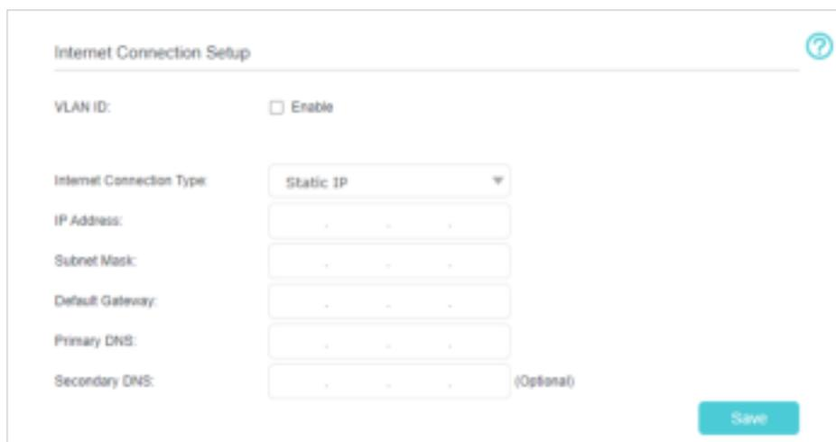
The screenshot shows the 'Internet Connection Setup' page with 'Static IP' selected in the 'Internet Connection Type' dropdown. Below this, there are input fields for 'IP Address', 'Subnet Mask', 'Default Gateway', 'Primary DNS', and 'Secondary DNS'. The 'Secondary DNS' field is marked as '(Optional)'. A 'Save' button is located at the bottom right of the form.
