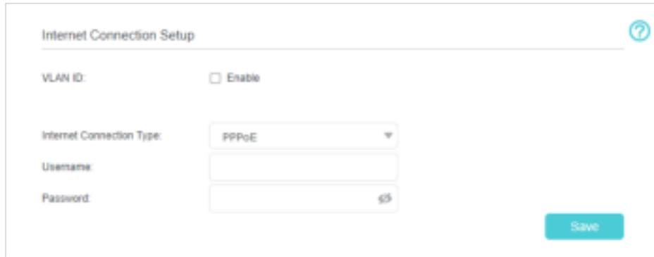
The screenshot shows the 'Internet Connection Setup' form. At the top right is a help icon. The form includes a 'VLAN ID' section with an 'Enable' checkbox. Below that is the 'Internet Connection Type' dropdown menu, which is set to 'PPPoE'. There are input fields for 'Username' and 'Password' (with a copy icon). A 'Save' button is located at the bottom right.
