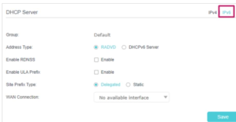
The screenshot shows the 'DHCP Server' configuration interface for IPv6. The 'Address Type' is set to 'RADVD' (selected with a radio button), and 'Enable RDNSS' and 'Enable ULA Prefix' are unchecked. The 'Site Prefix Type' is set to 'Delegated' (selected with a radio button). The 'WAN Connection' dropdown menu shows 'No available interface'. A 'Save' button is located at the bottom right of the form.
