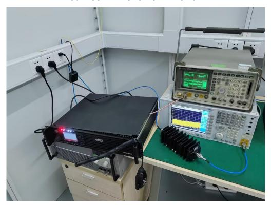
RADIATED EMISSION TEST SETUP BELOW 1GHz BY DC POWER
