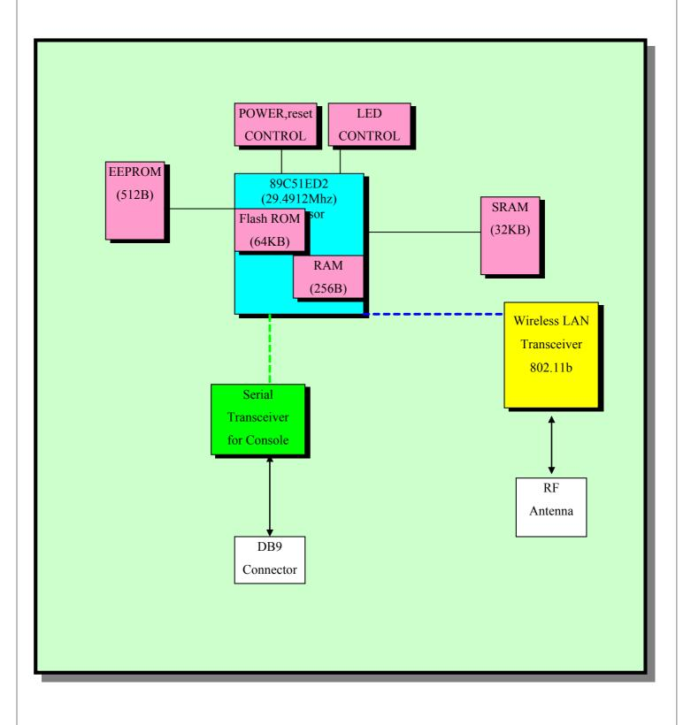
The LS100W uses Atmega 89C51ED2 CPU that is based on 8051 core specifications, and supports one Console/Serial port, and one 802.11b interface.
