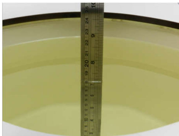
Fig 10.1 Photo of Liquid Height for Body SAR
