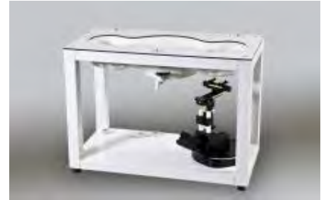
Figure 3.5.1 SAM Twin Phantom
