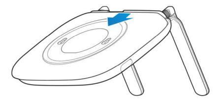
Insert the battery by aligning the metal contacts on the battery with the metal contacts in the battery compartment. Gently push down on the battery until it clicks into place.
