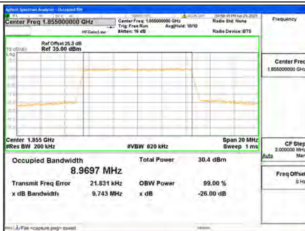
Band25 / 10MHz / 16QAM/ Low CH
