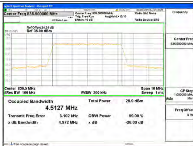
Band5 / 5MHz / 16QAM/ Mid CH
