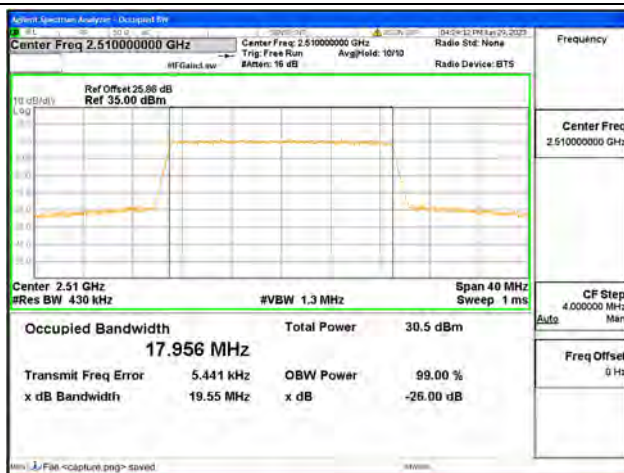
Band7 / 20MHz / 16QAM/ Low CH
