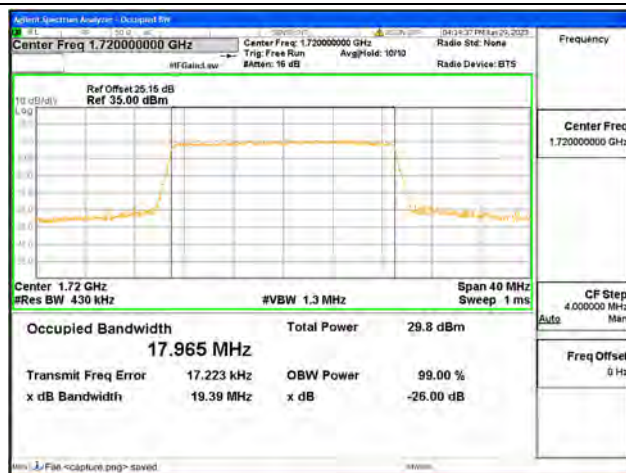
Band4 / 20MHz / 16QAM/ Low CH
