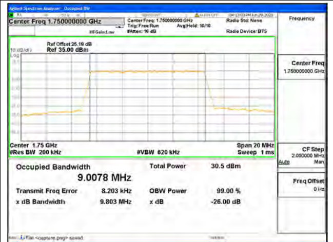
Band4 / 10MHz / QPSK/ High CH
