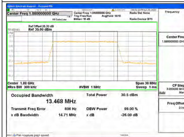
Band2 / 15MHz / 16QAM/ Mid CH
