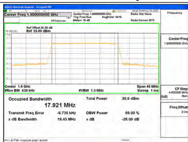
Band2 / 20MHz / 64QAM/ High CH
