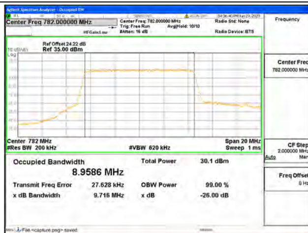
Band13 / 10MHz / 16QAM/ Mid CH
