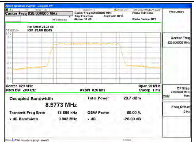
Band5 / 10MHz / 64QAM/ Low CH
