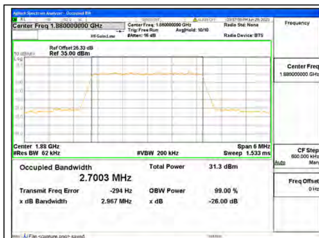
Band2 / 3MHz / QPSK/ Mid CH
