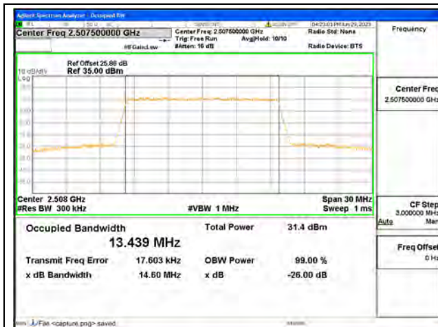
Band7 / 15MHz / QPSK/ Low CH
