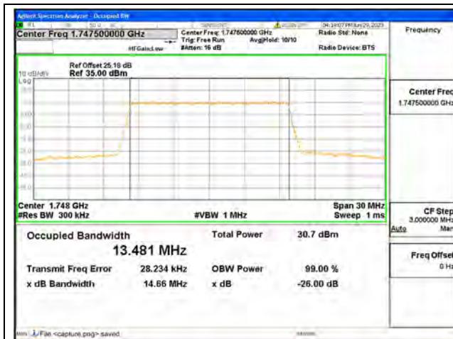
Band4 / 15MHz / QPSK/ High CH
