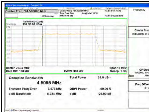
Band13 / 5MHz / QPSK/ High CH
