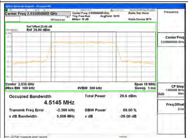
Band7 / 5MHz / 64QAM/ Mid CH
