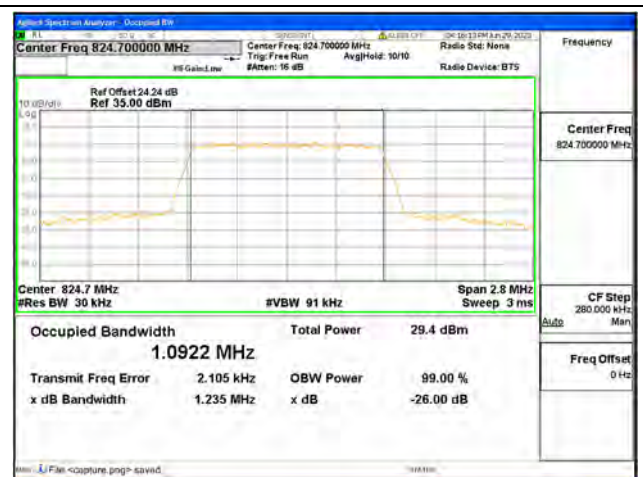
Band5 / 1.4MHz / 16QAM/ Low CH
