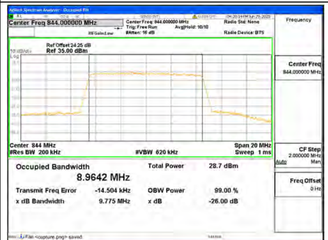
Band5 / 10MHz / 64QAM/ High CH
