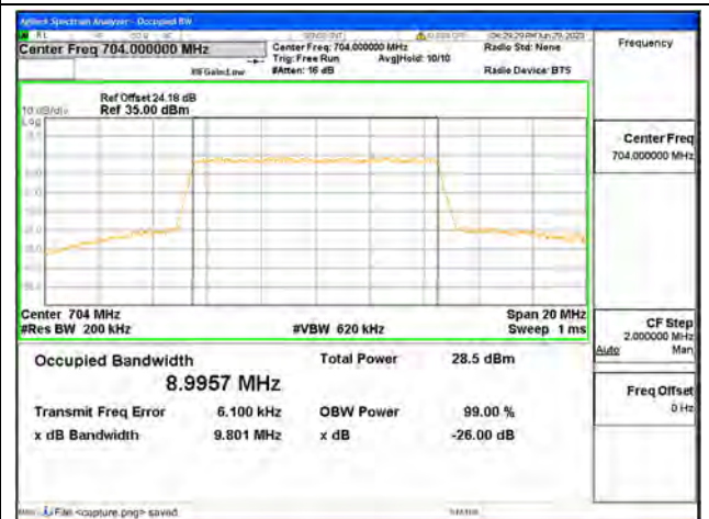
Band12 / 10MHz / 64QAM/ Low CH
