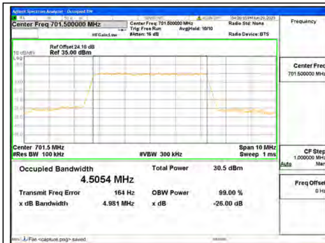
Band12 / 5MHz / QPSK/ Low CH
