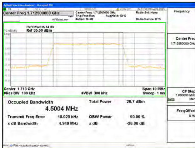
Band4 / 5MHz / 64QAM/ Low CH
