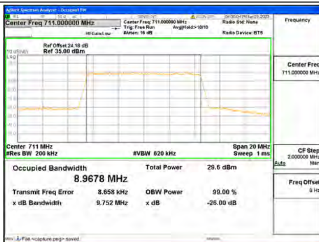
Band12 / 10MHz / 16QAM/ High CH
