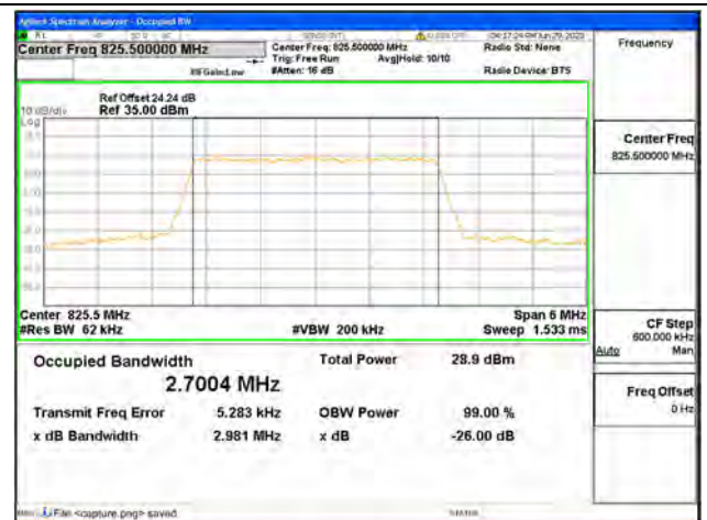
Band5 / 3MHz / 64QAM/ Low CH
