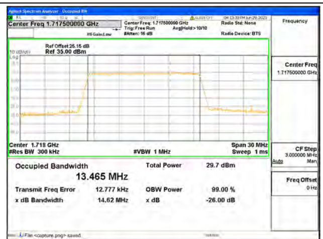
Band4 / 15MHz / 16QAM/ Low CH
