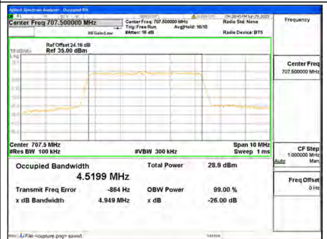
Band12 / 5MHz / 64QAM/ Mid CH
