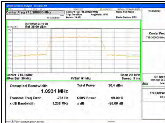
Band12 / 1.4MHz / QPSK/ High CH
