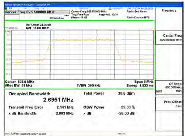
Band5 / 3MHz / QPSK/ Low CH
