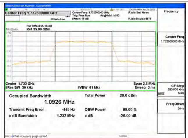
Band4 / 1.4MHz / 64QAM/ Mid CH
