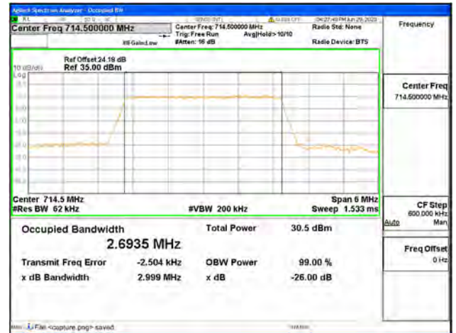
Band12 / 3MHz / QPSK/ High CH
