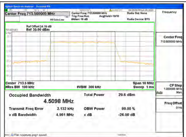
Band12 / 5MHz / 16QAM/ High CH
