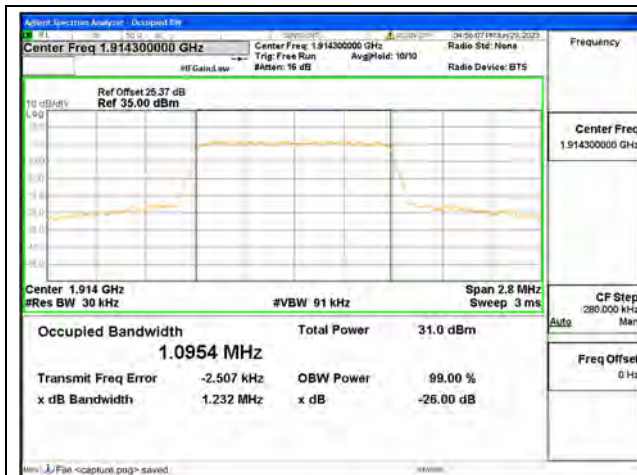
Band25 / 1.4MHz / QPSK/ High CH
