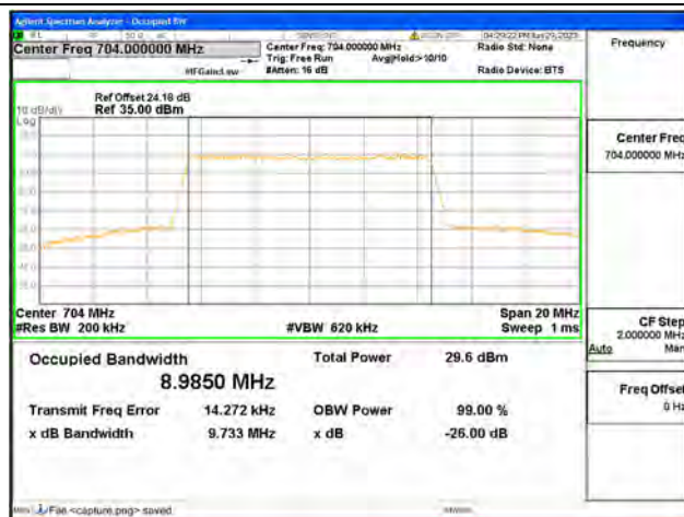
Band12 / 10MHz / 16QAM/ Low CH
