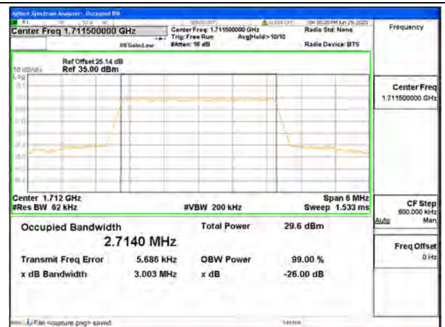
Band4 / 3MHz / 64QAM/ Low CH
