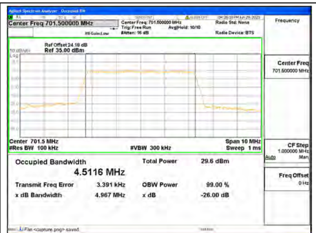
Band12 / 5MHz / 16QAM/ Low CH
