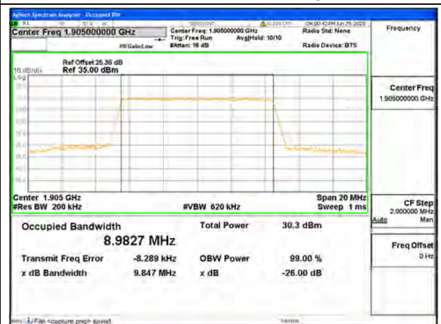
Band2 / 10MHz / 64QAM / High CH
