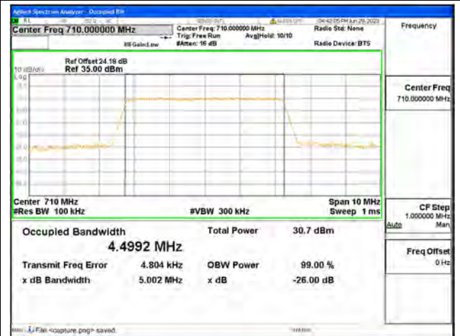
Band17 / 5MHz / QPSK/ Mid CH
