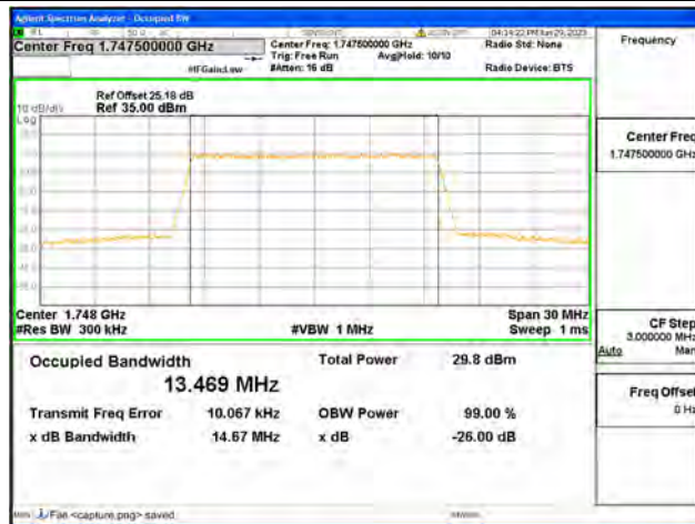
Band4 / 15MHz / 64QAM/ High CH
