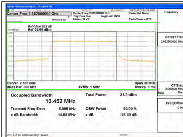
Band7 / 15MHz / QPSK/ High CH
