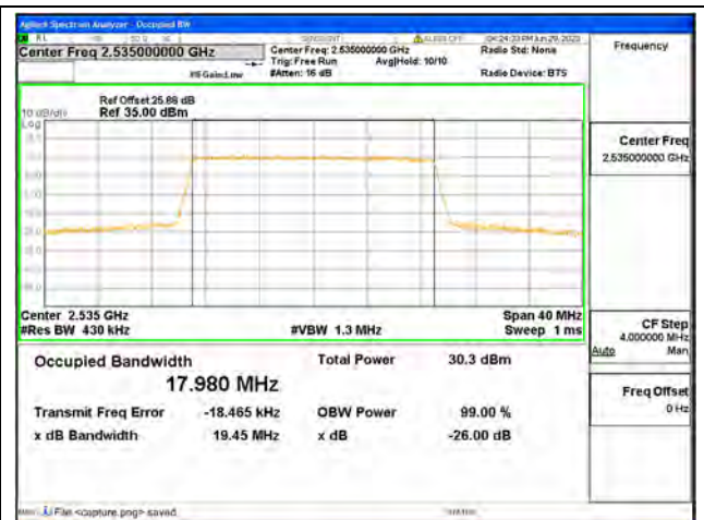
Band7 / 20MHz / 16QAM/ Mid CH
