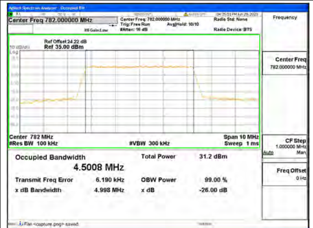
Band13 / 5MHz / QPSK/ Mid CH
