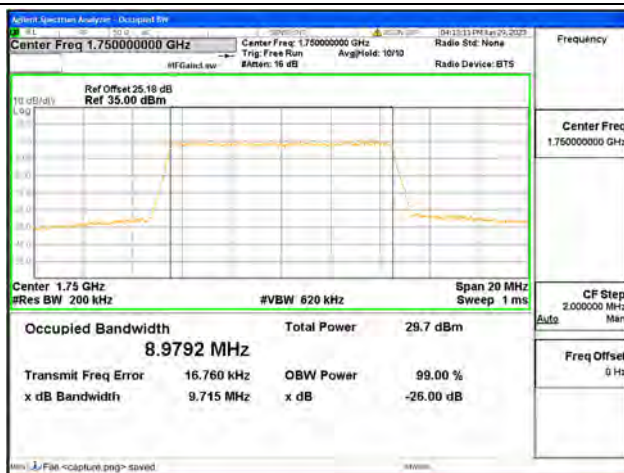
Band4 / 10MHz / 16QAM/ High CH
