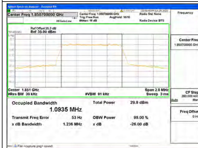
Band2 / 1.4MHz / 64QAM/ Low CH
