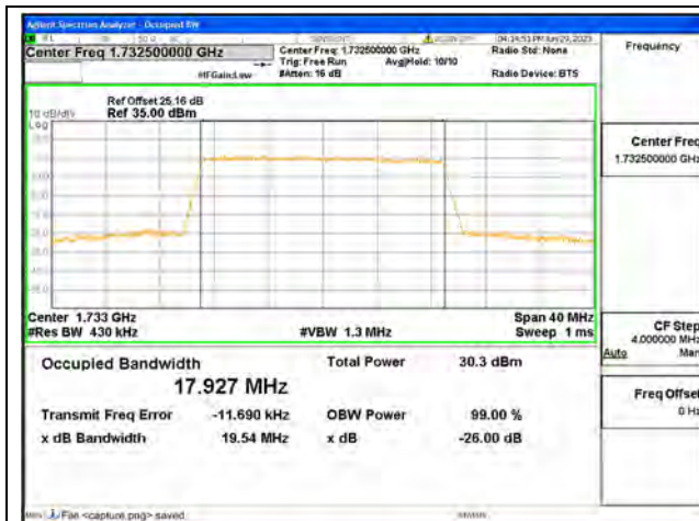
Band4 / 20MHz / QPSK/ Mid CH
