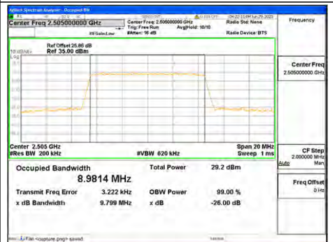
Band7 / 10MHz / 64QAM/ Low CH
