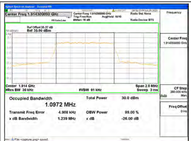
Band25 / 1.4MHz / 16QAM/ High CH
