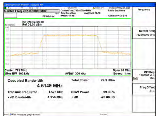
Band13 / 5MHz / 64QAM/ Mid CH
