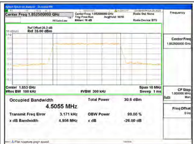
Band2 / 5MHz / 16QAM/ Low CH
