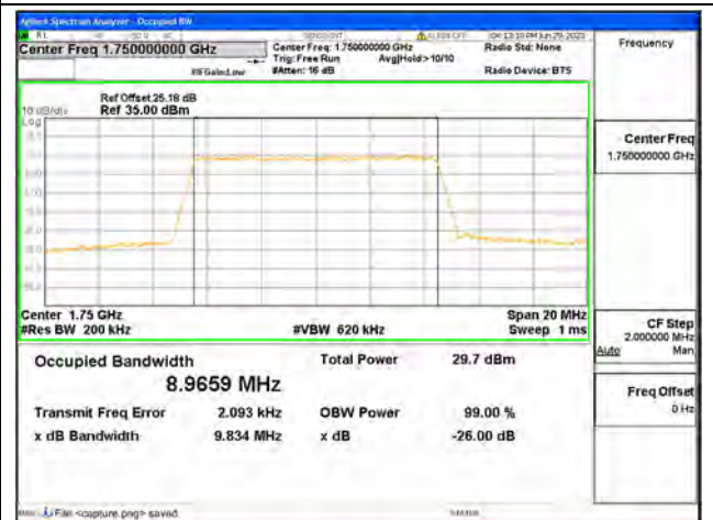
Band4 / 10MHz / 64QAM/ High CH
