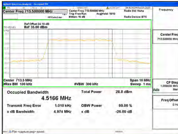
Band17 / 5MHz / 64QAM/ High CH
