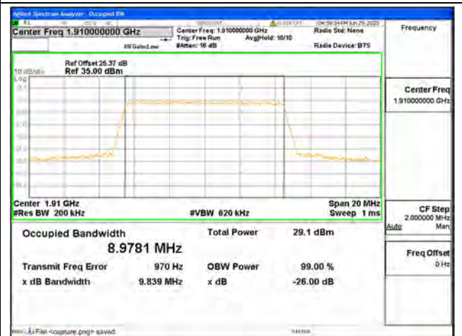
Band25 / 10MHz / 64QAM/ High CH
