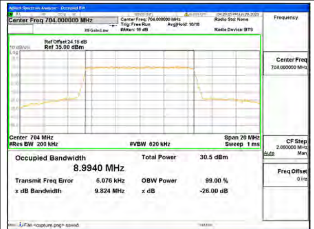
Band12 / 10MHz / QPSK/ Low CH
