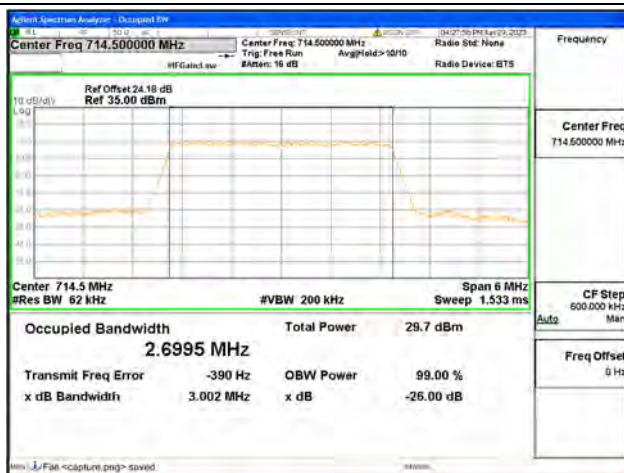
Band12 / 3MHz / 16QAM/ High CH
