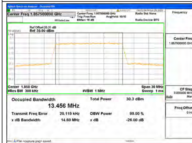
Band2 / 15MHz / 64QAM/ Low CH
