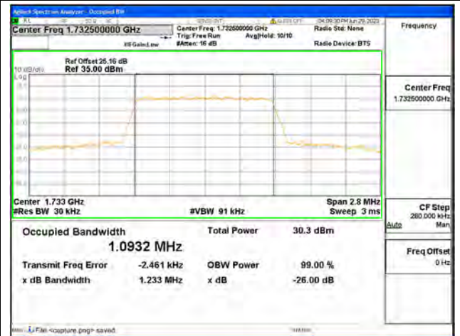
Band4 / 1.4MHz / QPSK/ Mid CH
