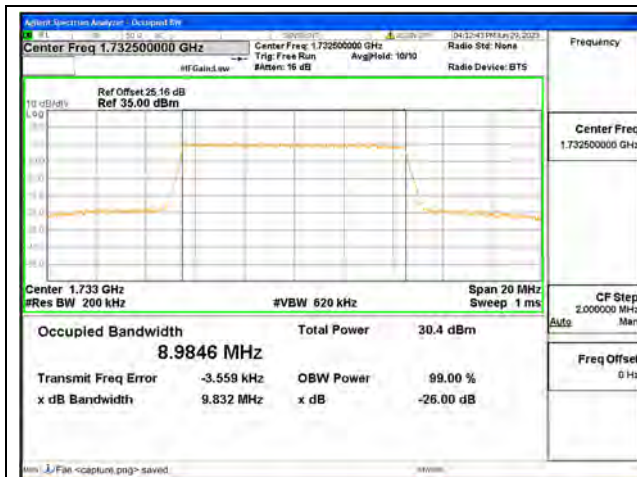
Band4 / 10MHz / QPSK/ Mid CH
