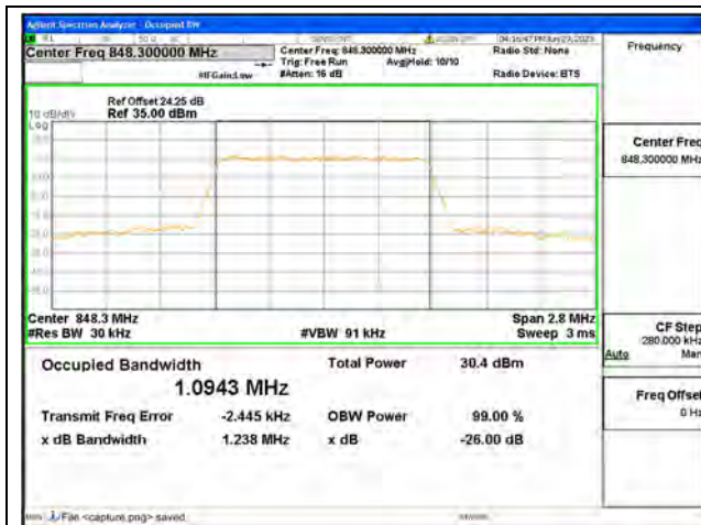
Band5 / 1.4MHz / QPSK/ High CH
