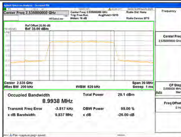
Band7 / 10MHz / 64QAM/ Mid CH
