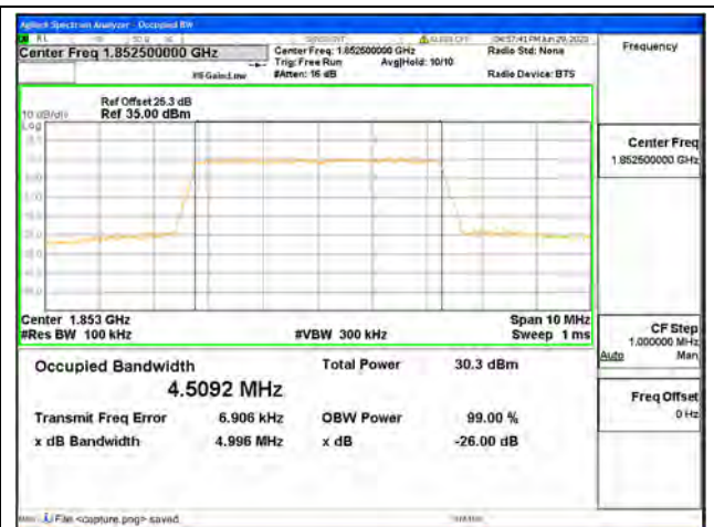
Band25 / 5MHz / 16QAM/ Low CH
