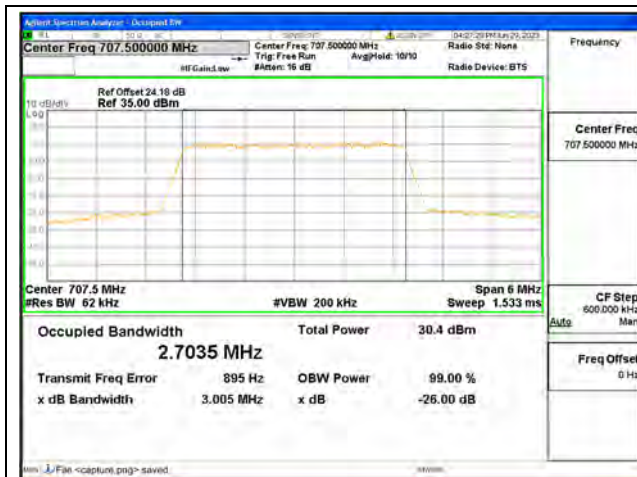
Band12 / 3MHz / QPSK/ Mid CH
