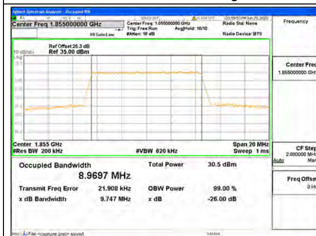
Band2 / 10MHz / 16QAM/ Low CH
