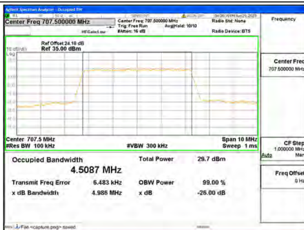
Band12 / 5MHz / 16QAM/ Mid CH
