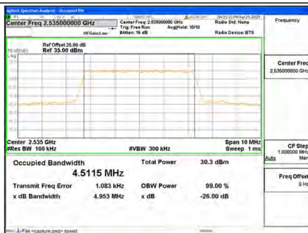
Band7 / 5MHz / 16QAM/ Mid CH
