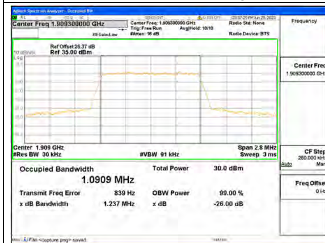
Band2 / 1.4MHz / 64QAM/ High CH
