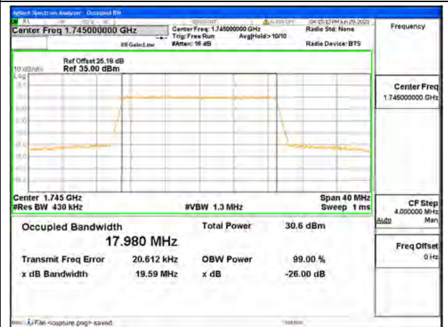
Band4 / 20MHz / QPSK/ High CH
