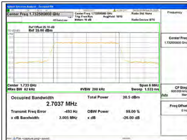
Band4 / 3MHz / QPSK/ Mid CH
