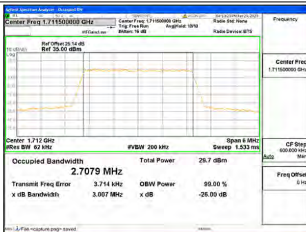
Band4 / 3MHz / 16QAM/ Low CH
