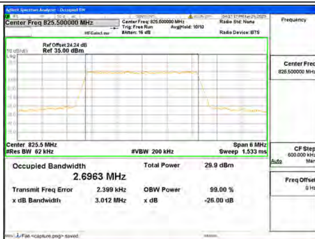
Band5 / 3MHz / 16QAM/ Low CH
