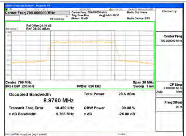
Band17 / 10MHz / 64QAM/ Low CH
