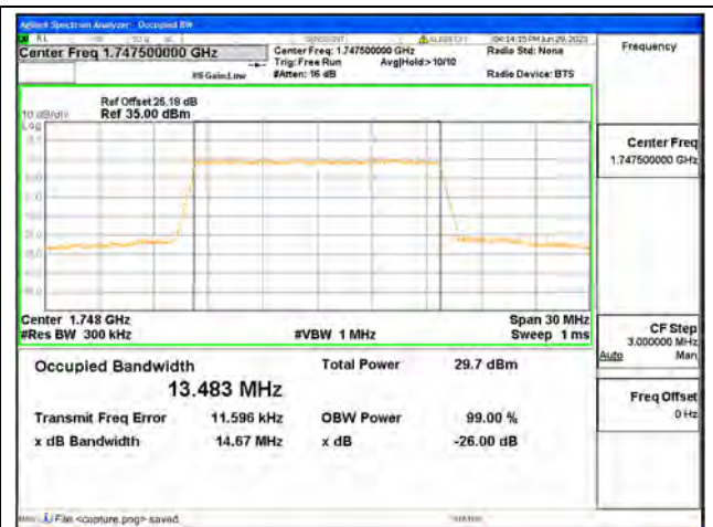
Band4 / 15MHz / 16QAM/ High CH
