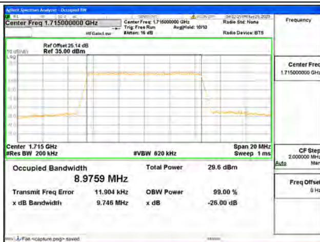
Band4 / 10MHz / 16QAM/ Low CH
