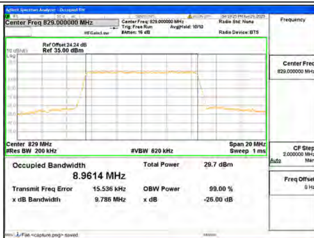
Band5 / 10MHz / 16QAM/ Low CH
