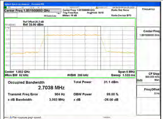
Band25 / 3MHz / QPSK/ Low CH
