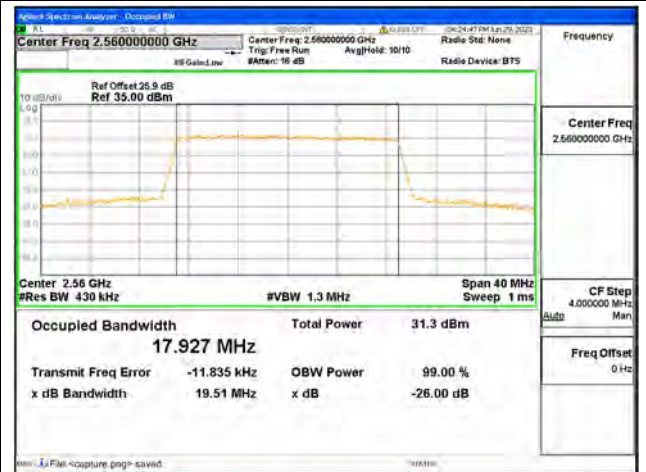
Band7 / 20MHz / QPSK/ High CH
