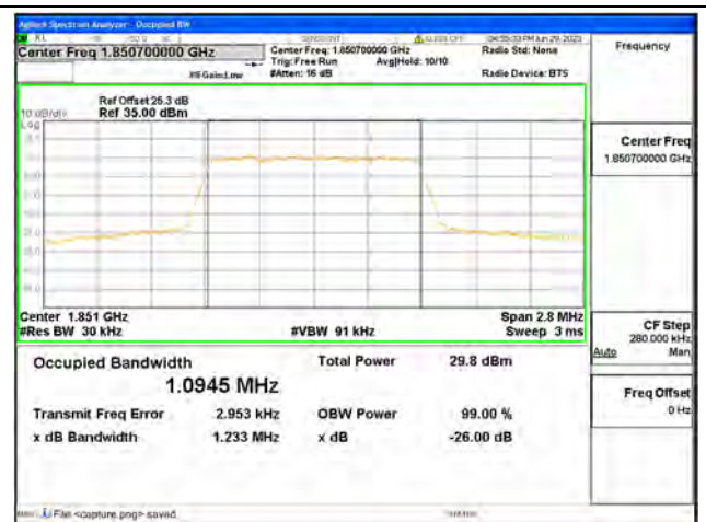
Band25 / 1.4MHz / 16QAM/ Low CH
