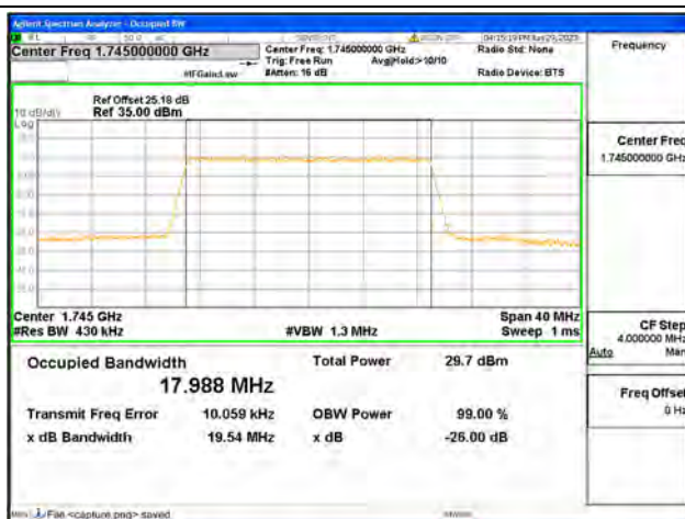
Band4 / 20MHz / 16QAM/ High CH
