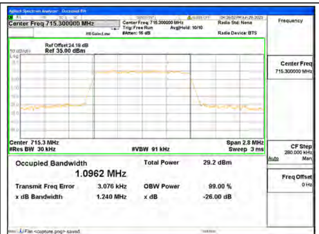
Band12 / 1.4MHz / 16QAM/ High CH
