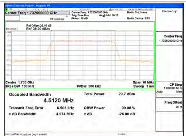
Band4 / 5MHz / 64QAM/ Mid CH
