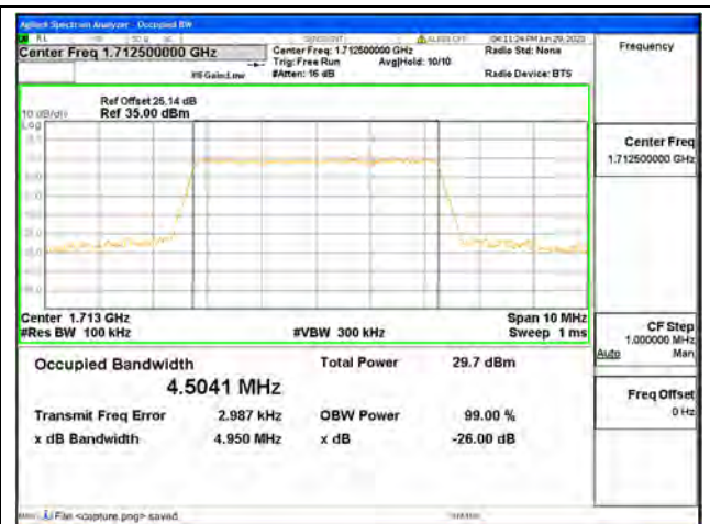
Band4 / 5MHz / 16QAM/ Low CH
