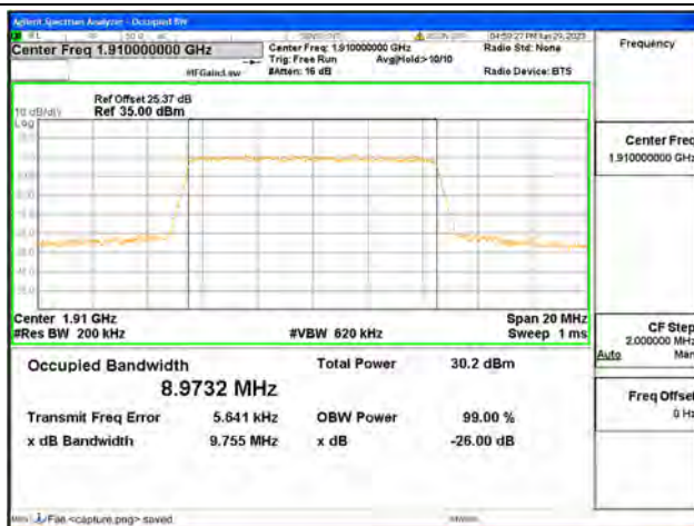
Band25 / 10MHz / 16QAM/ High CH
