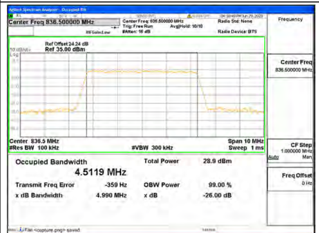
Band5 / 5MHz / 64QAM/ Mid CH
