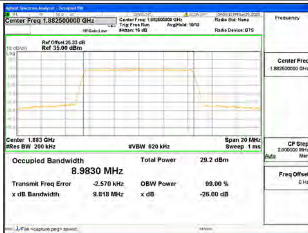
Band25 / 10MHz / 64QAM/ Mid CH
