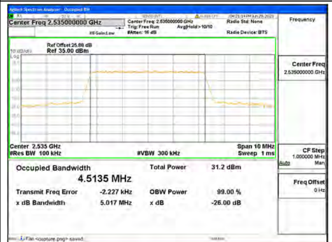
Band7 / 5MHz / QPSK/ Mid CH
