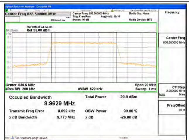
Band5 / 10MHz / 16QAM/ Mid CH
