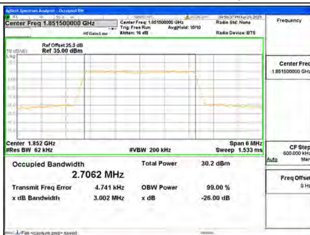
Band25 / 3MHz / 16QAM/ Low CH
