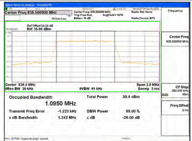
Band5 / 1.4MHz / QPSK/ Mid CH
