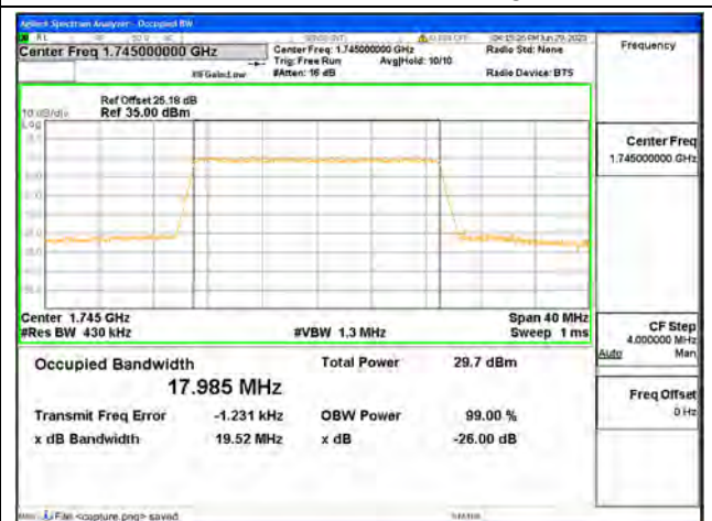
Band4 / 20MHz / 64QAM/ High CH
