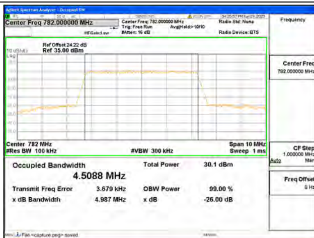
Band13 / 5MHz / 16QAM/ Mid CH
