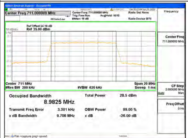
Band12 / 10MHz / 64QAM/ High CH
