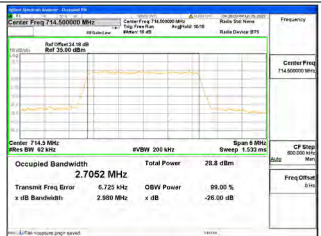
Band12 / 3MHz / 64QAM/ High CH
