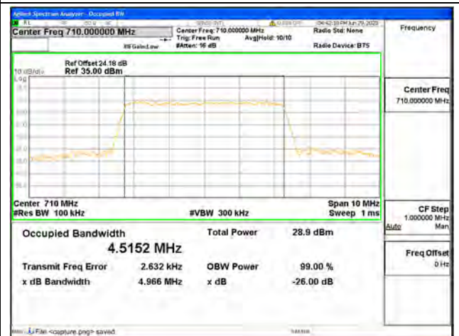
Band17 / 5MHz / 64QAM/ Mid CH
