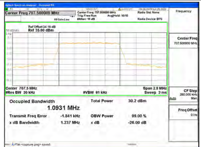
Band12 / 1.4MHz / QPSK/ Mid CH
