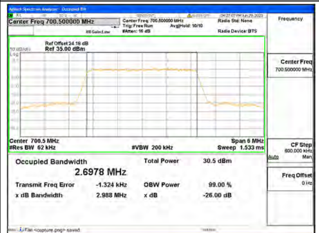
Band12 / 3MHz / QPSK/ Low CH
