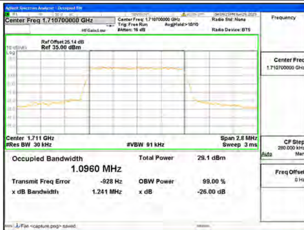
Band4 / 1.4MHz / 64QAM/ Low CH
