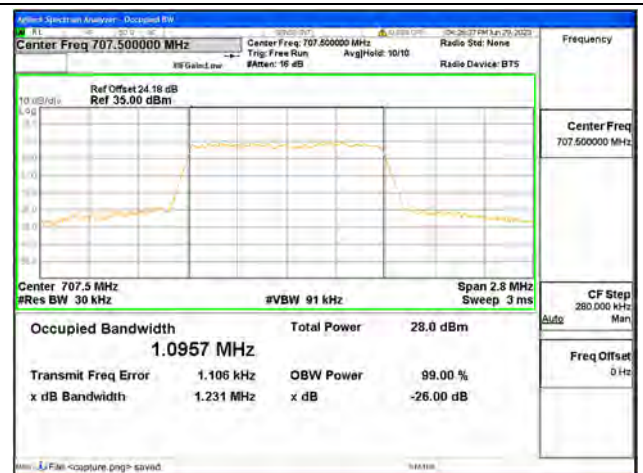
Band12 / 1.4MHz / 64QAM/ Mid CH
