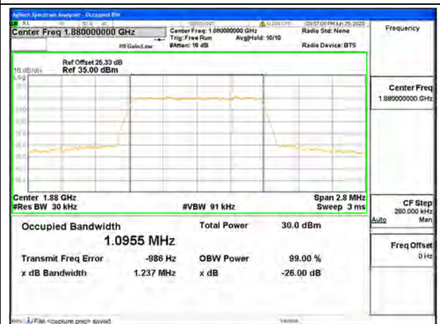
Band2 / 1.4MHz / 64QAM/ Mid CH
