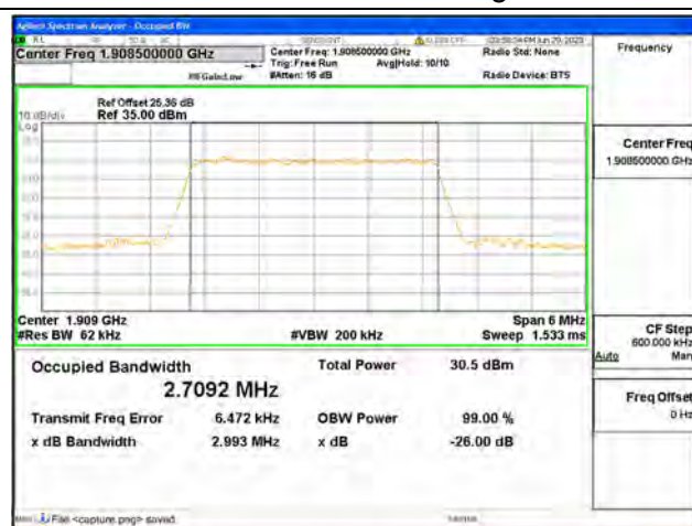
Band2 / 3MHz / 64QAM/ High CH
