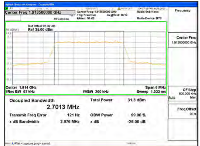
Band25 / 3MHz / QPSK/ High CH
