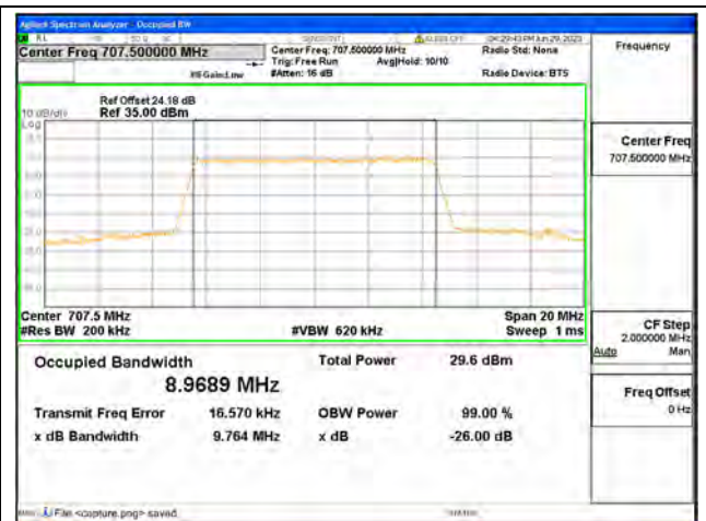
Band12 / 10MHz / 16QAM/ Mid CH
