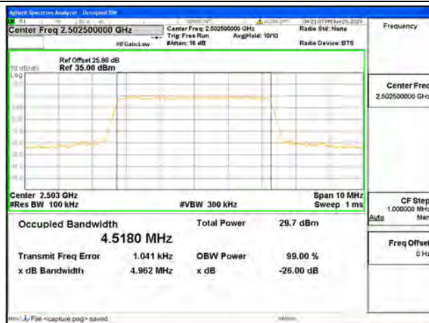
Band7 / 5MHz / 64QAM/ Low CH
