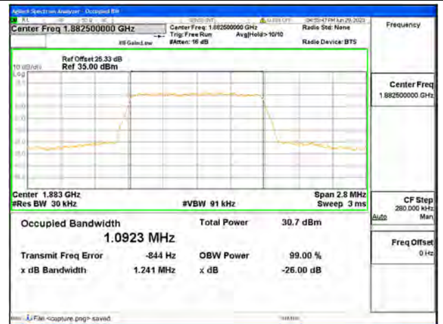
Band25 / 1.4MHz / QPSK/ Mid CH
