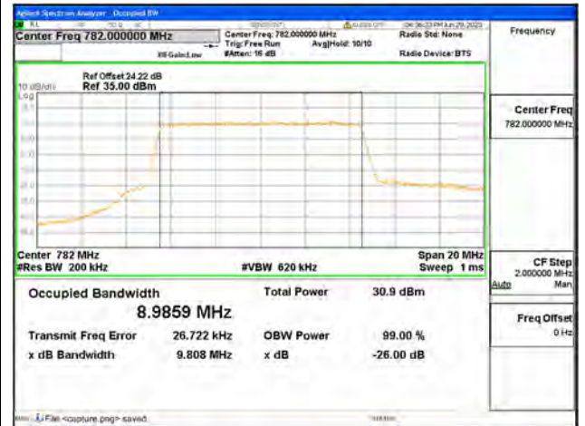
Band13 / 10MHz / QPSK/ Mid CH
