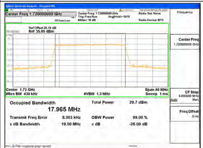
Band4 / 20MHz / 64QAM/ Low CH
