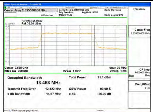
Band7 / 15MHz / QPSK/ Mid CH
