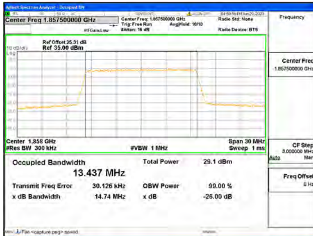
Band25 / 15MHz / 64QAM/ Low CH
