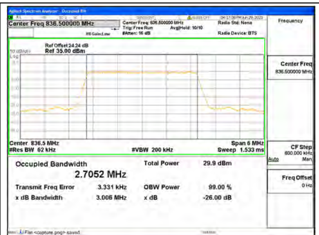
Band5 / 3MHz / 16QAM/ Mid CH
