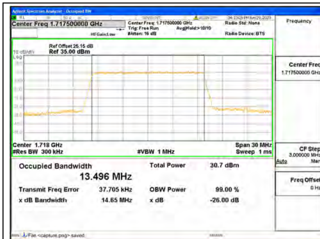
Band4 / 15MHz / QPSK/ Low CH
