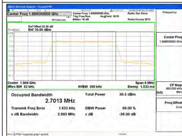
Band2 / 3MHz / 16QAM/ High CH
