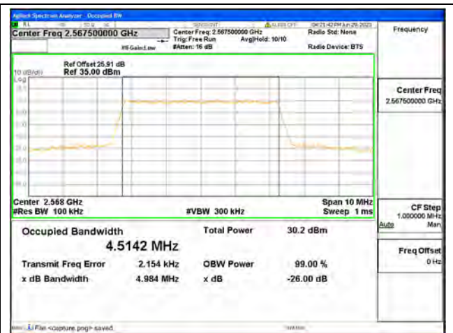
Band7 / 5MHz / 16QAM/ High CH
