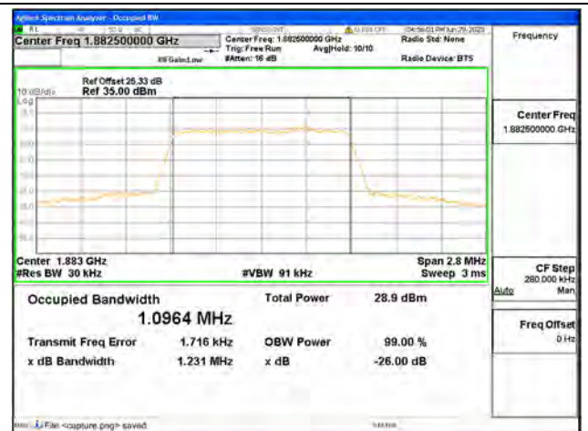
Band25 / 1.4MHz / 64QAM/ Mid CH
