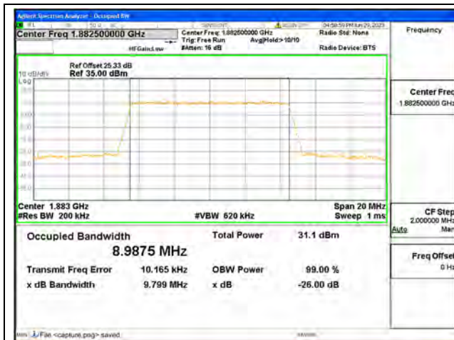
Band25 / 10MHz / QPSK/ Mid CH
