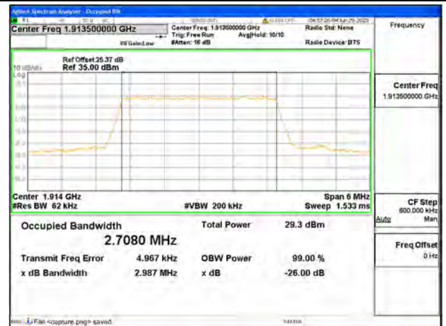
Band25 / 3MHz / 64QAM/ High CH
