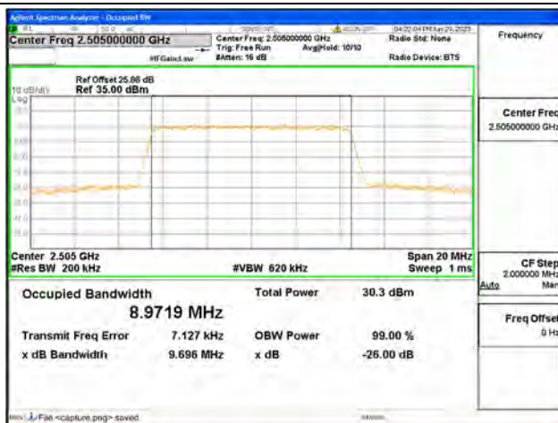
Band7 / 10MHz / 16QAM/ Low CH
