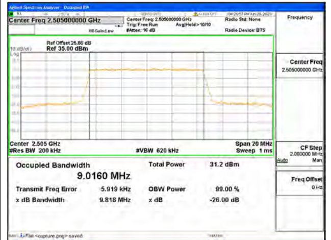
Band7 / 10MHz / QPSK/ Low CH
