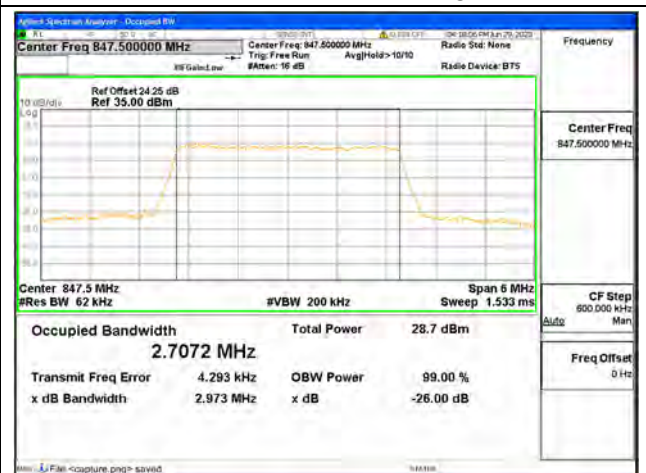
Band5 / 3MHz / 64QAM/ High CH
