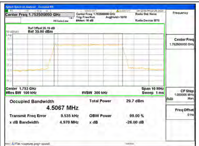
Band4 / 5MHz / 16QAM/ High CH
