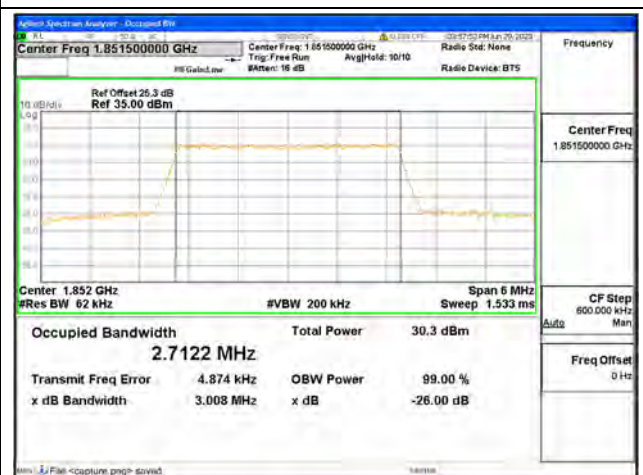
Band2 / 3MHz / 64QAM/ Low CH
