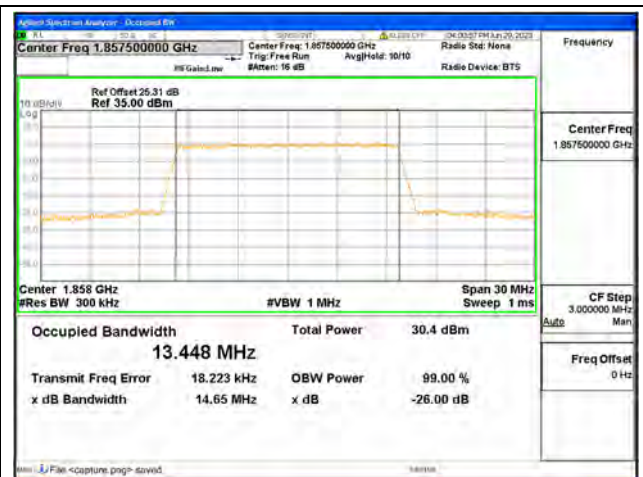
Band2 / 15MHz / 16QAM/ Low CH
