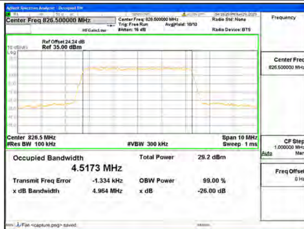
Band5 / 5MHz / 64QAM/ Low CH
