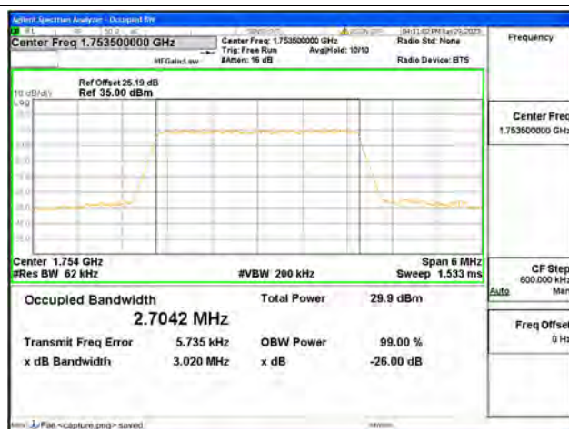
Band4 / 3MHz / 16QAM/ High CH
