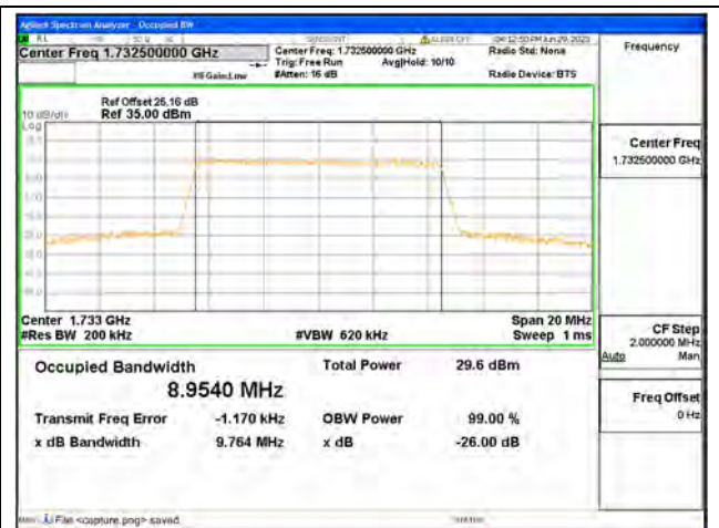
Band4 / 10MHz / 16QAM/ Mid CH
