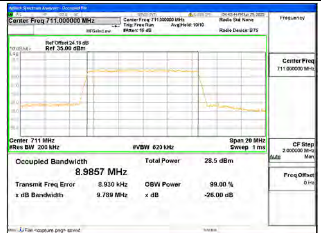
Band17 / 10MHz / 64QAM/ High CH
