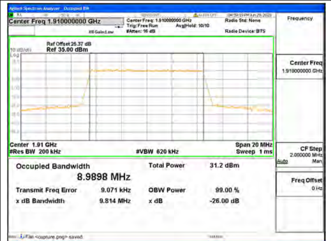
Band25 / 10MHz / QPSK/ High CH
