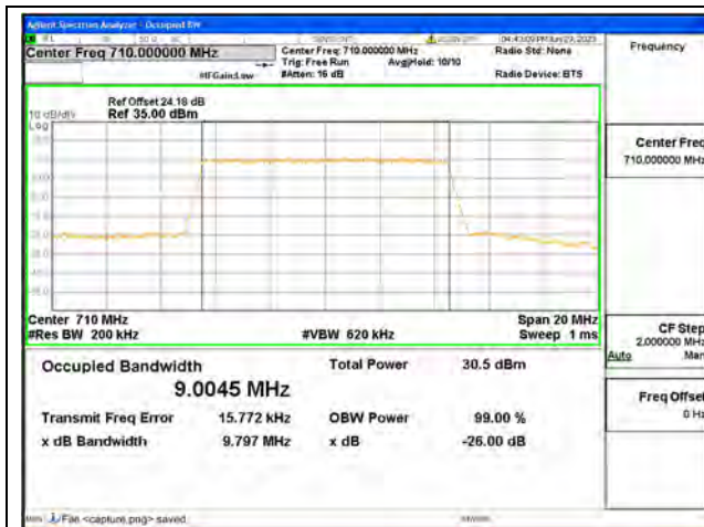
Band17 / 10MHz / QPSK/ Mid CH
