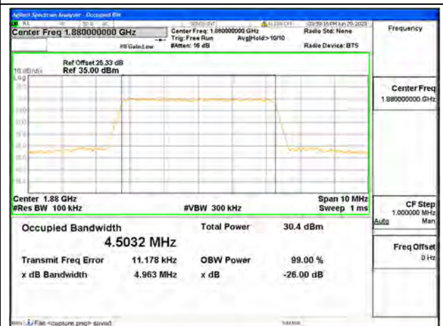
Band2 / 5MHz / 64QAM/ Mid CH
