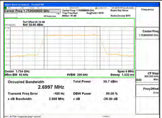
Band4 / 3MHz / QPSK/ High CH
