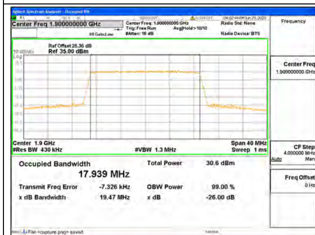
Band2 / 20MHz / 16QAM/ High CH
