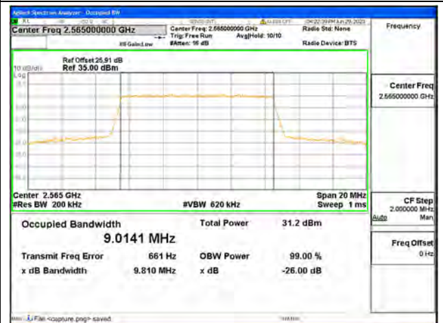
Band7 / 10MHz / QPSK/ High CH
