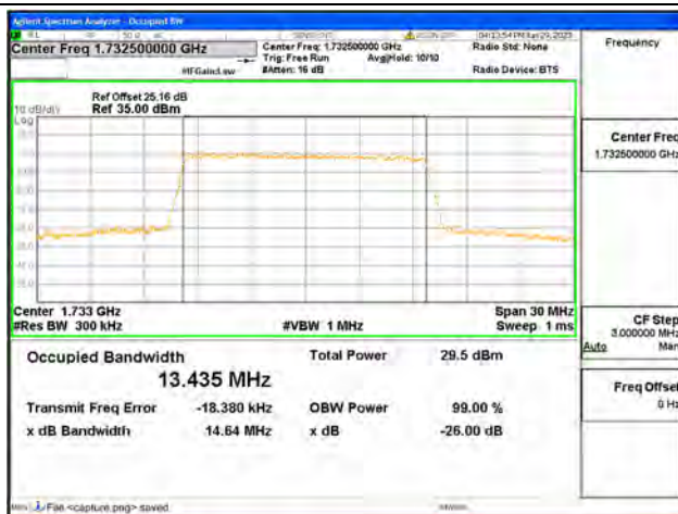
Band4 / 15MHz / 16QAM/ Mid CH
