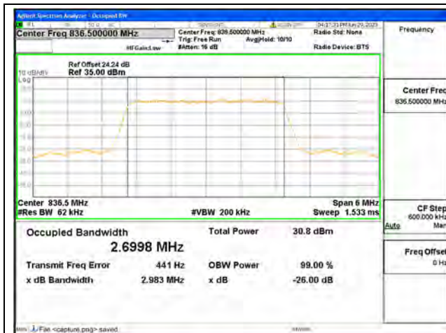
Band5 / 3MHz / QPSK/ Mid CH
