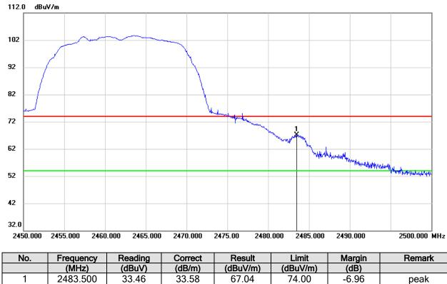
Note: 1. Measurement = Reading Level + Correct Factor.
