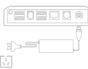
3. Connect the power interface of the adapter to the power port at the bottom of the mainframe. And insert the other side of the adapter to electric supply sockets
