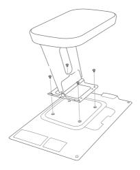
6. Unscrew the four M4 screws with a screwdriver and complete the removal of base.
