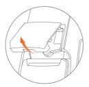
Firstly, open outward the cover of the printer cutter
