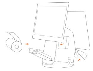
Pull the printer handle out, and the paper roller cover pops out automatically.
