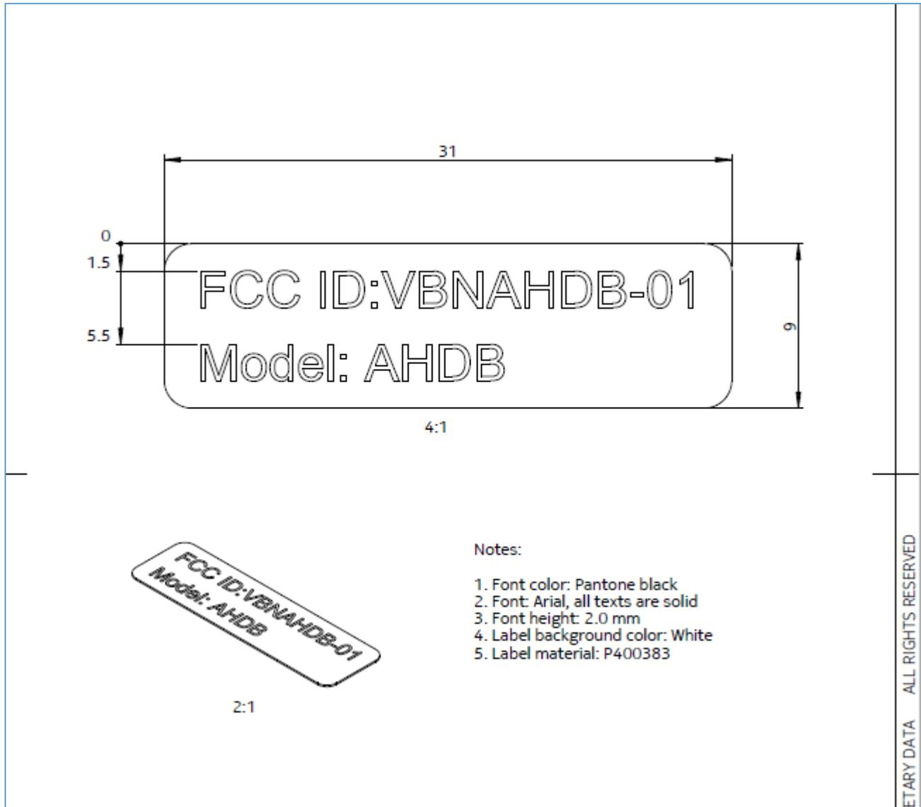
FCC Label Location for AHDB AirScale 2T4R B8 Sub-Band 160W, FCC ID: VBNAHDB-01
