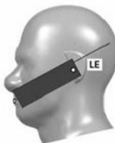
Picture14 Handset vertical and horizontal reference lines—"clam-shell case"
