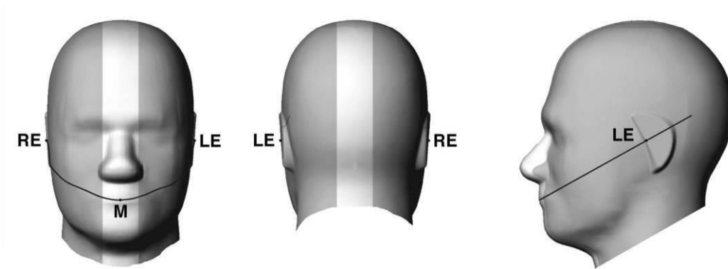
Picture10: Front, back, and side views of SAM twin phantom
